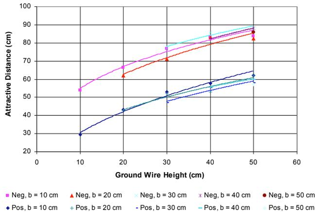
**Fig. (6).** Attractive distance of two ground wires for different ground wire separation width under negative and positive polarity,  $H = 73$  cm.
