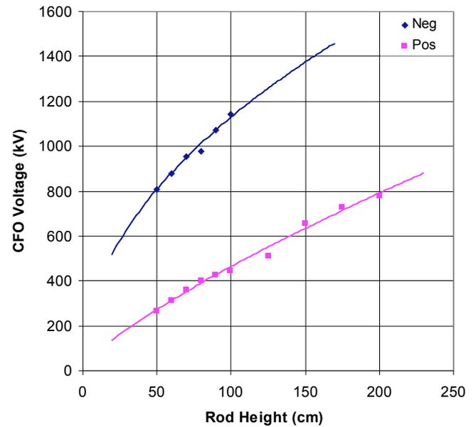
Fig. (4). Switching impulse CFO voltages of a rod-plane gap for negative and positive polarity.
