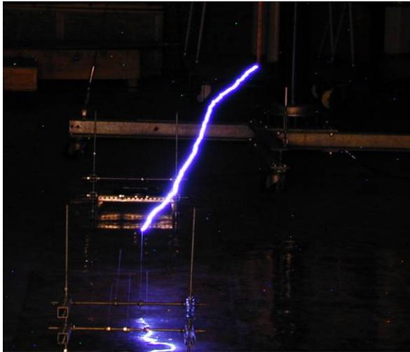
(c) Flash to the line, positive polarity.
