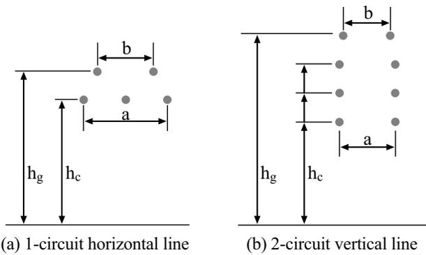
Fig. (3). Transmission line models ( $h_g$ : average ground wire height;  $h_c$ : average phase conductor height).
