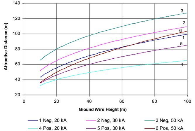
Fig. (11). Attractive distance as a function of ground wire height for different lightning stroke current.
