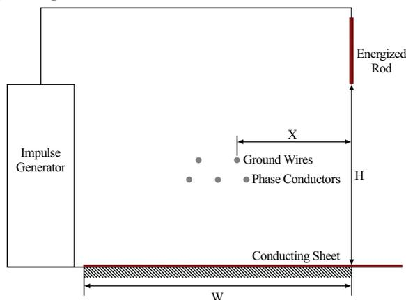
**Fig. (1).** Diagram of the test system for the study ( $X$ : attractive distance;  $W$ : attractive width;  $H$ : rod height).
