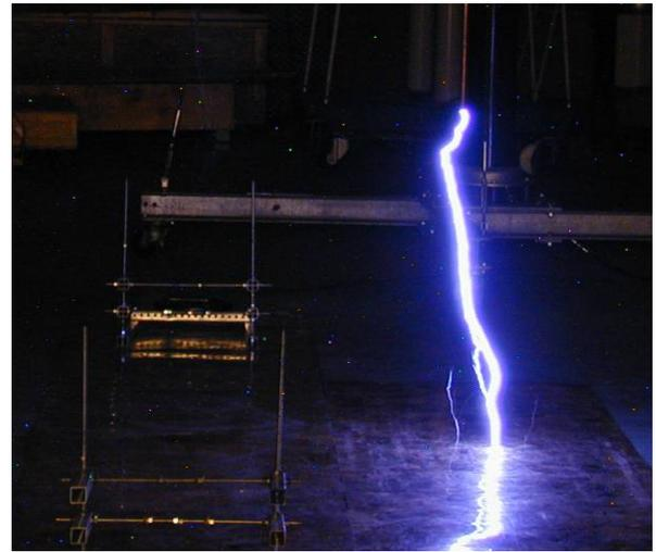
(b) Flash to the ground, negative polarity.
