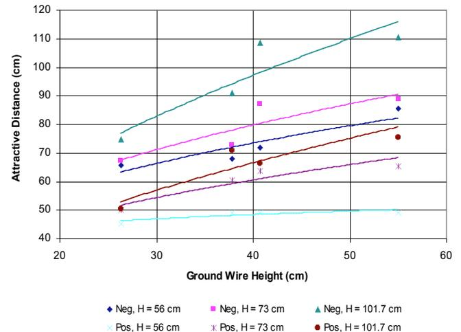
**Fig. (8).** Attractive distance of double-circuit vertical lines for different rod heights under negative and positive polarity.
