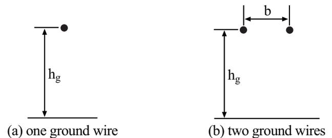
**Fig. (2).** Models of overhead ground wires.
