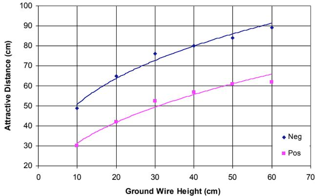
**Fig. (5).** Attractive distance of one ground wire under negative and positive polarity,  $H = 73$  cm.
