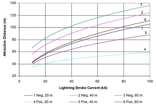
Fig. (12). Attractive distance as a function of lightning stroke current for different ground wire height.
