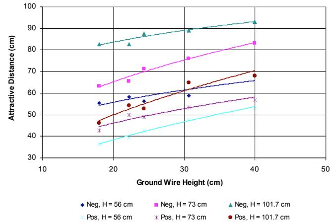
**Fig. (7).** Attractive distance of single-circuit horizontal lines for different rod heights under negative and positive polarity.
