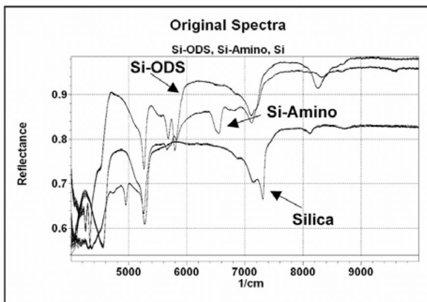
Fig. (4). Original NIR spectra of raw, octadecylated and amino derivatised silica. Conditions: Wavenumber range, 4500 - 9996  $\text{cm}^{-1}$ ; scans, ten; temperature, 23  $^{\circ}\text{C}$ .
