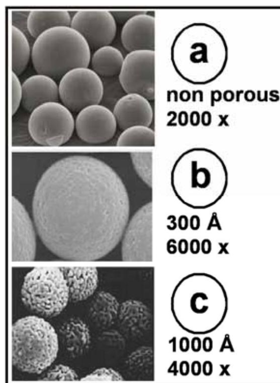
**Fig. (2).** Scanning electron micrograph (SEM) pictures of (a) non-porous (1.5 µm), (b) 300 Å (5 µm) and (c) 1000 Å (7 µm) particles.
