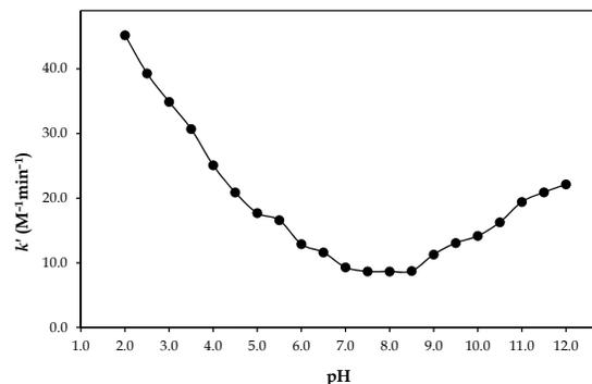
**Fig. (2).**  $k'$ -pH profile for the photolysis of cyanocobalamin in the presence of riboflavin.
