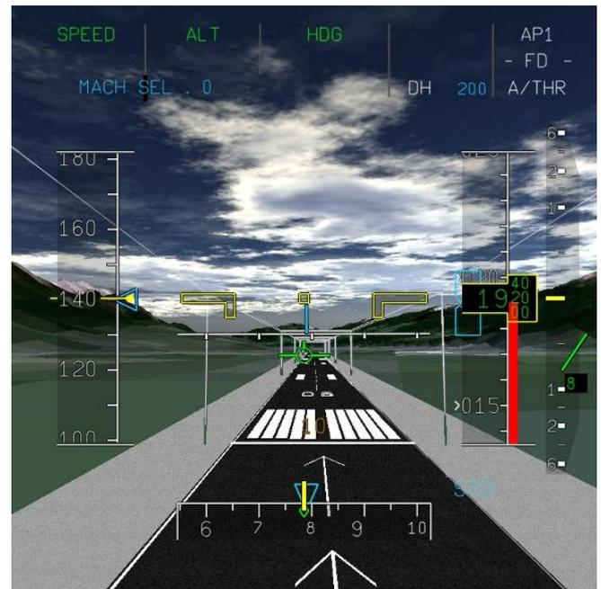
Fig. (7). Synthetic vision display with textures and FPV (D5).
