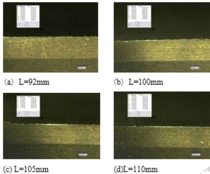
Fig. (1). Results of milling cutter flank face wear.
