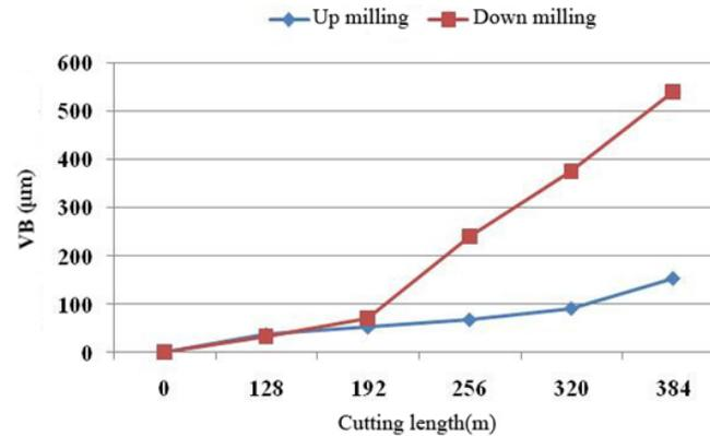
**Fig. (4).** Wear curve comparison between down and up milling.
