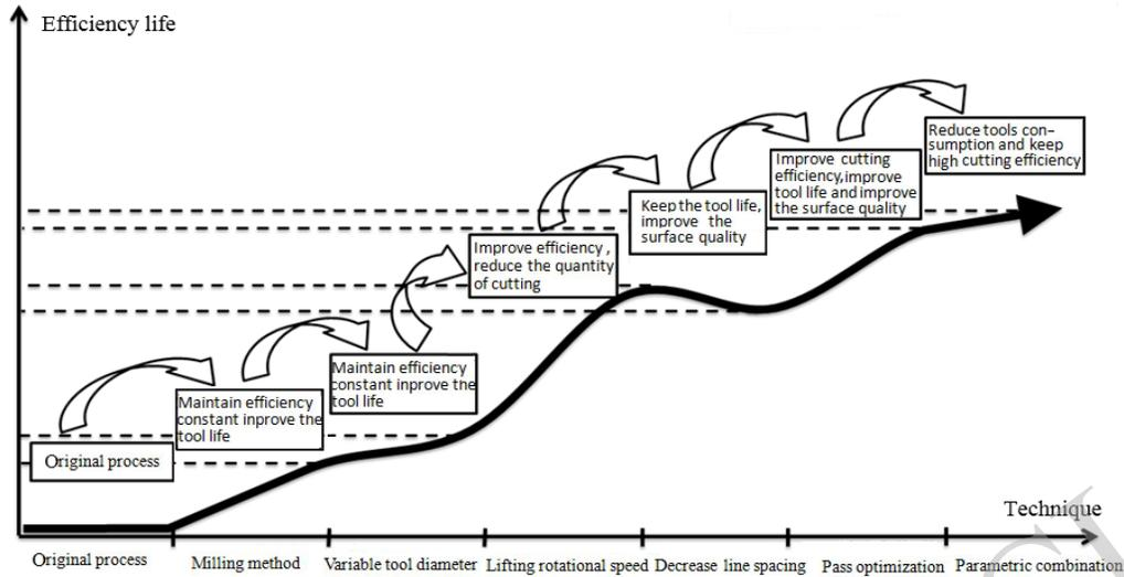
Fig. (7). Process of controlling cutter consumption.
