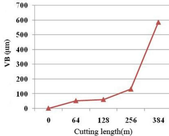
Fig. (5). Wear curve of fixed-angle cutting.
