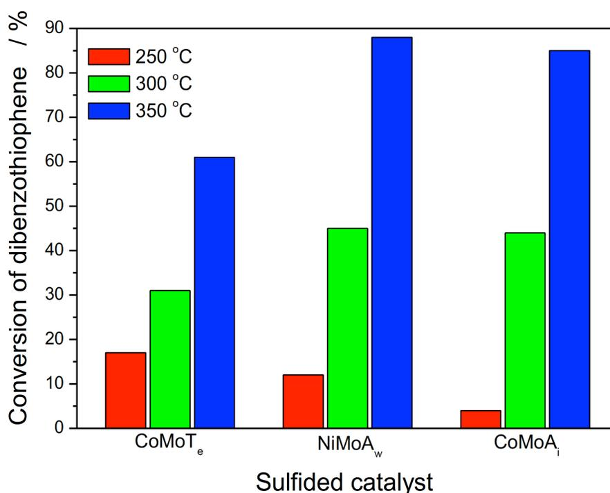
**Fig. (4).** Conversion of dibenzothiophene over selected sulfided catalysts upon simultaneous HDO and HDS tests (W= 0.2 g, F= 0.25 ml/min, Feed composition: 1% wt. phenol and 1% wt. dibenzothiophene in hexadecane, P= 15 bar).
