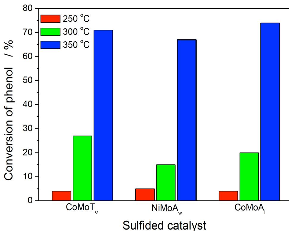
**Fig. (3).** Conversion of phenol over selected sulfided catalysts upon simultaneous HDO and HDS tests (W= 0.2 g, F=0.25 ml/min, Feed composition: 1% phenol and 1% dibenzothiophene in hexadecane, P= 15 bar).
