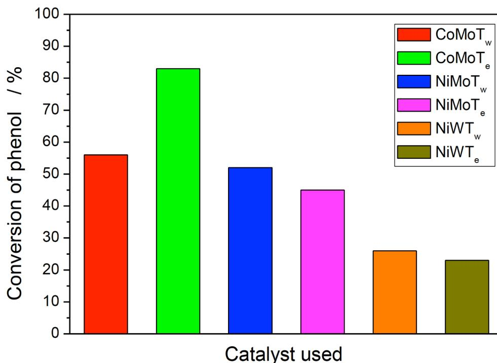
**Fig. (2).** Conversion of phenol over reduced wet impregnated and EDF catalysts supported on titania (W= 0.2 g, F=0.25 ml/min, T= 350°C, P= 15 bar).
