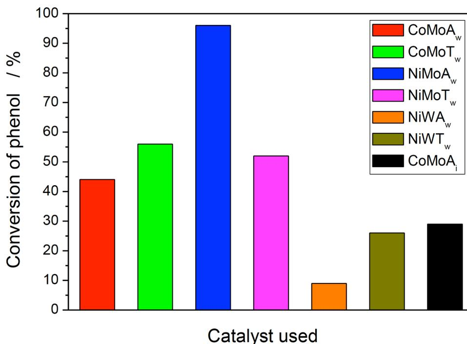
**Fig. (1).** Conversion of phenol over reduced wet impregnated catalysts supported on alumina and titania ( $W = 0.2$  g,  $F = 0.25$  ml/min,  $T = 350^\circ\text{C}$ ,  $P = 15$  bar).
