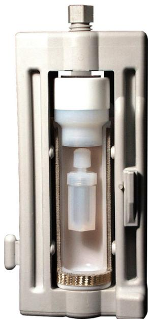
**Fig. (1).** Control MicroVessel™ (7 mL) assembly inserted inside an HP-500 Plus control vessel.
