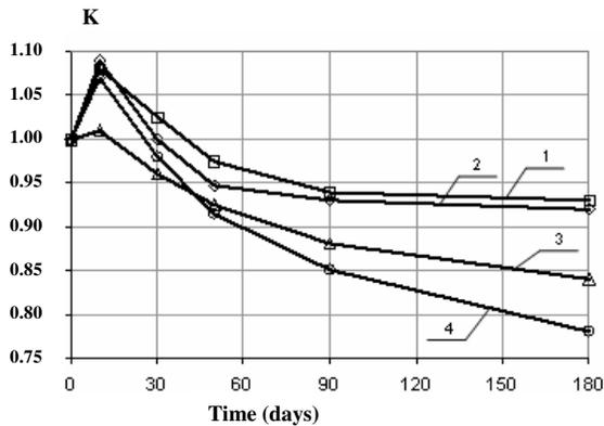
**Fig. (7).** The coefficient chemical resistance dependence of the exposure time; 1 - 70 %- solution of  $H_2SO_4$ ; 2 - 5 %- solution of  $H_3PO_4$ ; 3 - 25 %- solution of  $NH_4OH$ ; 4 - 36 %- solution of  $HCl$ .
