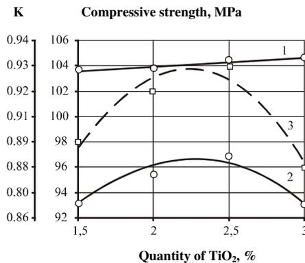
**Fig. (4).** Impact of TiO<sub>2</sub> quantity on *RubCon* compressive strength operated in no aggressive environments (line 1), resistance coefficient (line 2) and compressive strength (line 3) after 90 days exposition into 36% solution of HCl.
