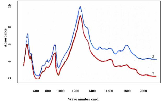
**Fig. (9).** Specters of *RubCon*: 1- before  $\gamma$ -exposition, 2- after  $\gamma$ -exposition.
