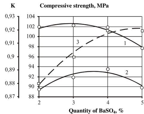
**Fig. (5).** Impact of BaSO<sub>4</sub> quantity on *RubCon* compressive strength operated in no aggressive environments (line 1), compressive strength (line 2) and resistance coefficient (line 3) after 90 day's exposition into 36% solution of HCl.
