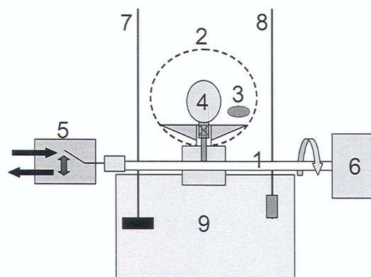
**Fig. (2).** Schematic representation of the dissolution stress test device (1) central axis ( $\varnothing$  8 mm), (2) chamber ( $\varnothing$  35 mm mesh size 0.5 mm, wire 0.1 mm), (3) dosage form, (4) inflatable balloon, (5) solenoid valves, (6) stepping motor, (7) stirrer (paddle 15x35 mm<sup>2</sup>), (8) sampling, (9) standard vessel (reproduced with permission from ref [60]).
