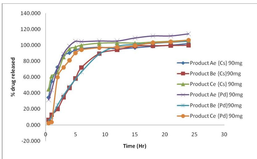
**Fig. (3).** Comparative dissolution profiles of diltiazem (120mg) Extended release tablets (n=6) with the crescent- shaped spindle {Cs} at 25rpm and the USP paddle spindle {Pd} at 100rpm.
