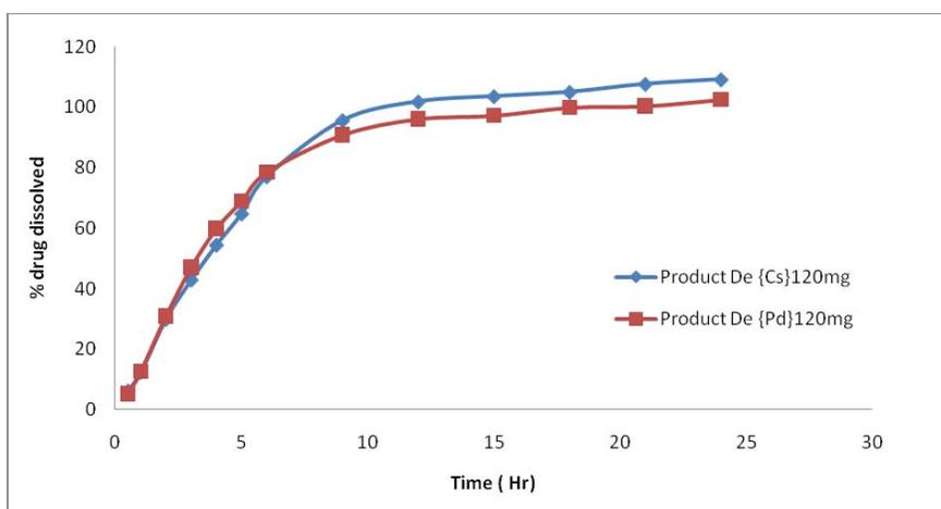
Fig. (4). Comparative dissolution profiles of diltiazem (120mg) extended release Capsules (n=6) with the crescent- shaped spindle {Cs} at 25rpm and the USP paddle spindle {Pd} at 100rpm.
