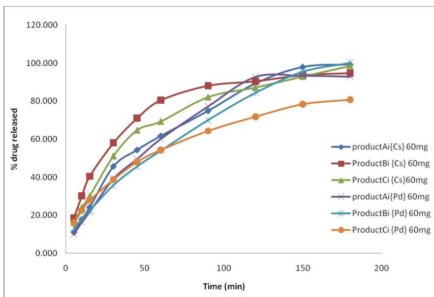
**Fig. (1).** Comparative dissolution profiles of diltiazem (60mg) Immediate release tablets (n=6) with the crescent- shaped spindle {Cs} at 25rpm and the USP paddle spindle {Pd} at 75rpm.
