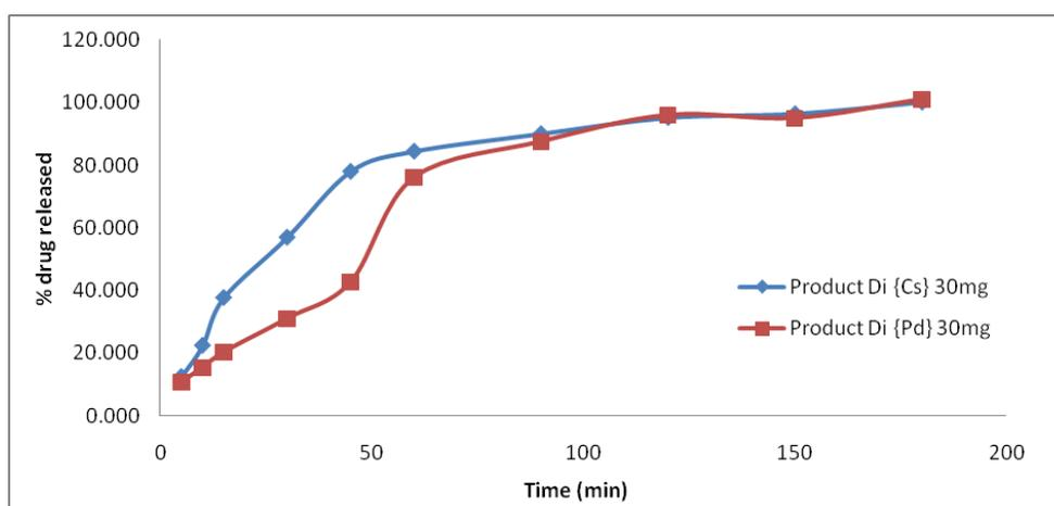
**Fig. (2).** Comparative dissolution profiles of diltiazem (30mg) Immediate release tablets (n=6) with the crescent- shaped spindle {Cs} at 25rpm and the USP paddle spindle {Pd} at 75rpm.
