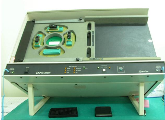
Fig. (1). An ESD test machine (KeyTek Zapmaster 7/4).
