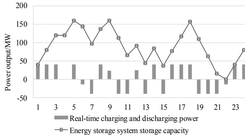
Fig. (2). Charge and discharge optimization result of energy storage system.
