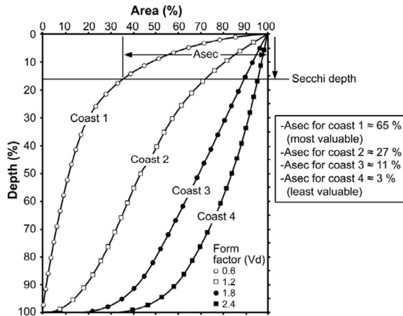
**Fig. (4).** Illustration of relative hypsographic curves that illustrates the depth-area relationship of four coastal areas with different shape (and form factor = volume development = Vd). The shape influences the area above the Secchi depth (Asec), which indicate the production capacity and “biological value” of the coastal system.
