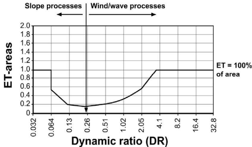
**Fig. (5).** The relation between the dynamic ratio (DR) and the proportion of bottom areas dominated by erosion and transport processes (ET). Redrawn from [41].
