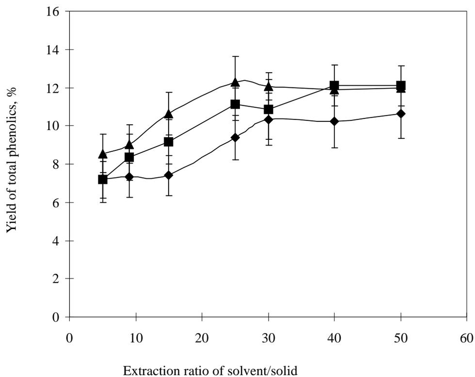
**Fig. (5).** The effect of the ratio of solvent /solid ( $\text{g}\cdot\text{g}^{-1}$ ) used in the extraction on the yield of total phenolics. The extraction time was 2 min and the particle size of 40 mesh was used.  $\blacklozenge$ , 25°C;  $\blacksquare$ , 60°C;  $\blacktriangle$ , 95°C.
