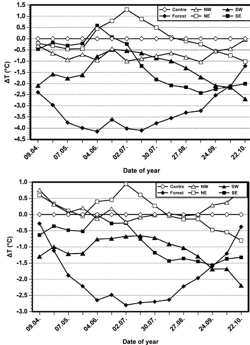
**Fig. (3c).** Seasonal course of mean daily maxima (above) and minima (below) of soil temperature at all measuring sites during the study period from April to October 2005. Values are plotted as deviations from the respective value at the central station  $\Delta T_i = T_i - T_{\text{Centre}}$ .
