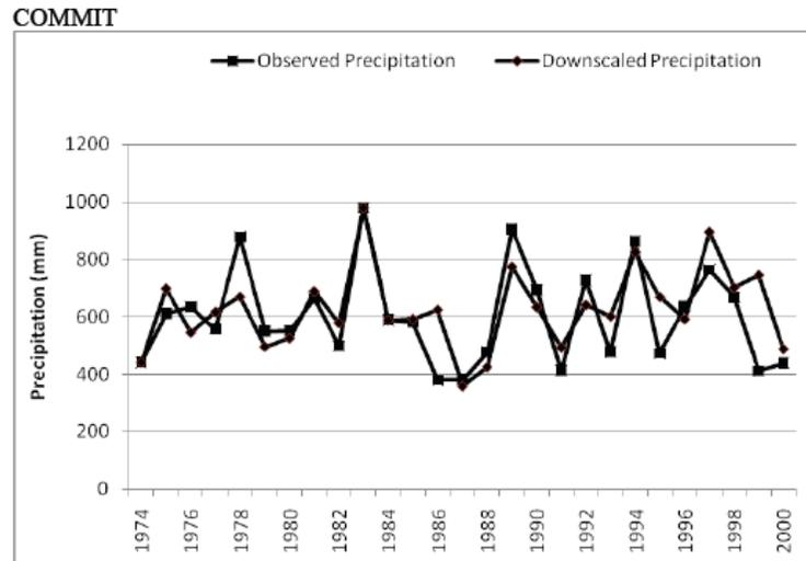
**Fig. (9).** Typical results for comparison of the mean annual observed precipitation with precipitation simulated using ANN downscaling model ANNM4 for NCEP data. In the figure, calibration period is from 1974 to 1994, and the rest is validation period.
