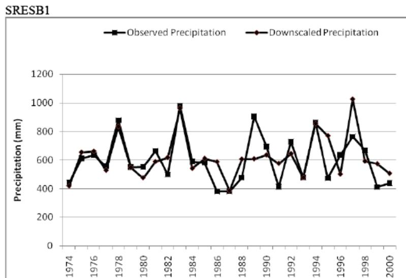
**Fig. (8).** Typical results for comparison of the mean annual observed precipitation with precipitation simulated using ANN downscaling model ANNM3 for NCEP data. In the figure, calibration period is from 1974 to 1994, and the rest is validation period.
