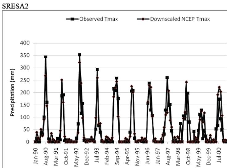
**Fig. (11).** Typical results for comparison of the amean monthly observed precipitation with precipitation simulated using ANN downscaling model ANNM6 for NCEP data. In the figure, calibration period is from January 1990 to December 1995, and the rest is validation period.
