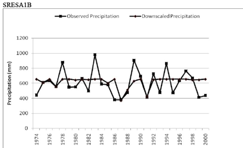
**Fig. (6).** Typical results for comparison of the mean annual observed precipitation with precipitation simulated using ANN downscaling model ANNM1 for NCEP data. In the figure, calibration period is from 1974 to 1994, and the rest is validation period.
