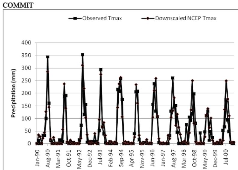
Fig. (13). Typical results for comparison of the amean monthly observed precipitation with precipitation simulated using ANN downscaling model ANNM8 for NCEP data. In the figure, calibration period is from January 1990 to December 1995, and the rest is validation period.
