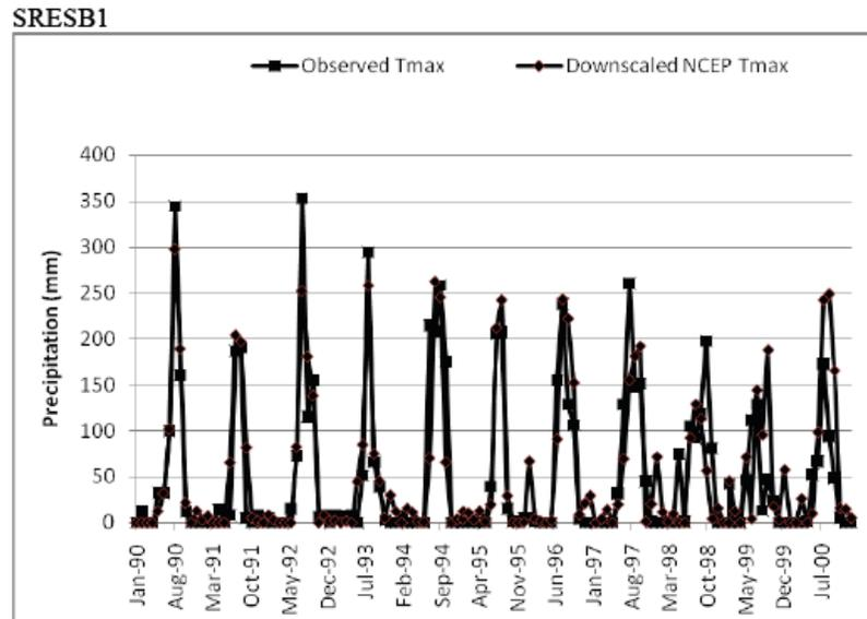
Fig. (12). Typical results for comparison of the amean monthly observed precipitation with precipitation simulated using ANN downscaling model ANNM7 for NCEP data. In the figure, calibration period is from January 1990 to December 1995, and the rest is validation period.
