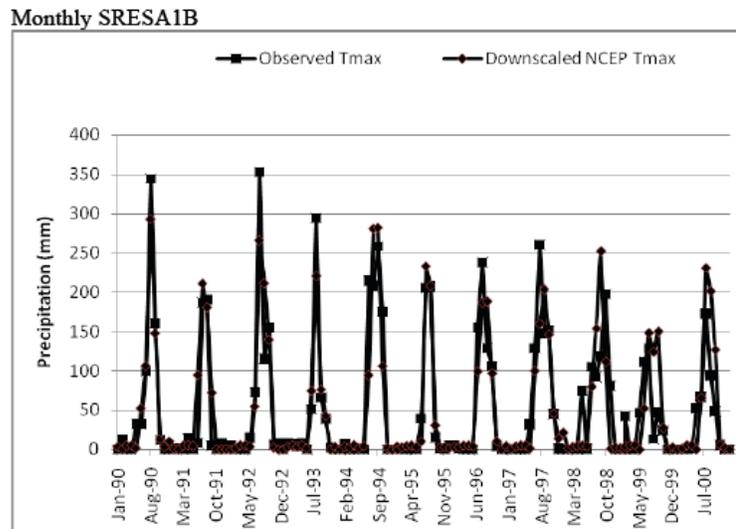
**Fig. (10).** Typical results for comparison of the amean monthly observed precipitation with precipitation simulated using ANN downscaling model ANNM5 for NCEP data. In the figure, calibration period is from January 1990 to December 1995, and the rest is validation period.
