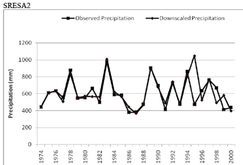
**Fig. (7).** Typical results for comparison of the mean annual observed precipitation with precipitation simulated using ANN downscaling model ANNM2 for NCEP data. In the figure, calibration period is from 1974 to 1994, and the rest is validation period.
