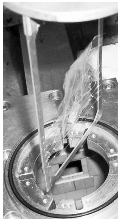
**Fig. (3).** SU-8 microturbine sample fastened with Teflon strings onto an aluminium frame for introduction into the PGAA measurement chamber.
