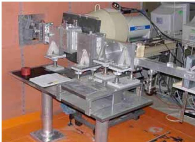
**Fig. (2).** The Prompt Gamma Activation Analysis Instrument at the BRR.
