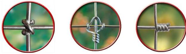
**Fig. (2).** Selection of knots used in the fabrication of rectangular netted wire fencing. From left: stiff-stay, fixed, and hinge-joint knot. Each knot has its own unique characteristics which see them used for different applications. These knots require dedicated tooling and hence consideration at the early stages of the design of the machine. (Image courtesy South Fence Machinery (New Zealand))
