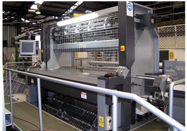
**Fig. (1).** Example of a specialised machine for knitting wire fences. Various knot types are available: this particular machine produces a fence with a 'stiff-stay' knot. The image hardly does justice to the size, complexity, and engineering precision of these specialised machines. This particular machine is designed and manufactured by South Fence Machinery (New Zealand). (Image used by permission of that firm).
