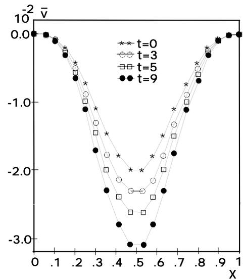
Fig. (2). Time response of circumferential displacement  $\bar{v}$  along  $X$ .
