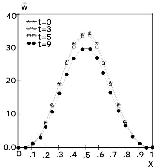
Fig. (3). Time response of normal displacement  $\bar{w}$  along  $X$ .
