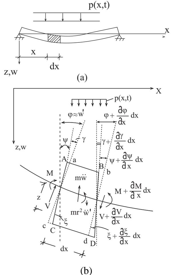
**Fig. (2).** The deformed state of the infinitesimal part  $dx$ .
