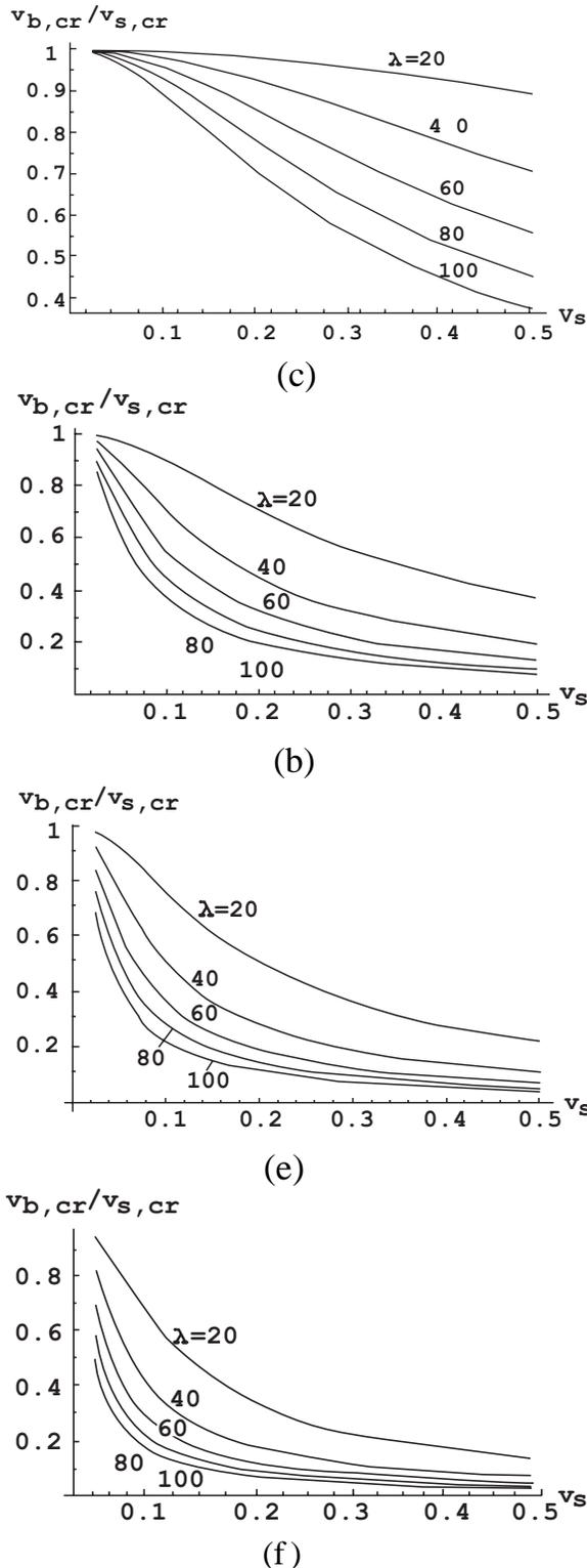
Fig. (8). Velocity ratio  $v_{b,cr}/v_{s,cr}$  vs soil speed  $v_s$ .
