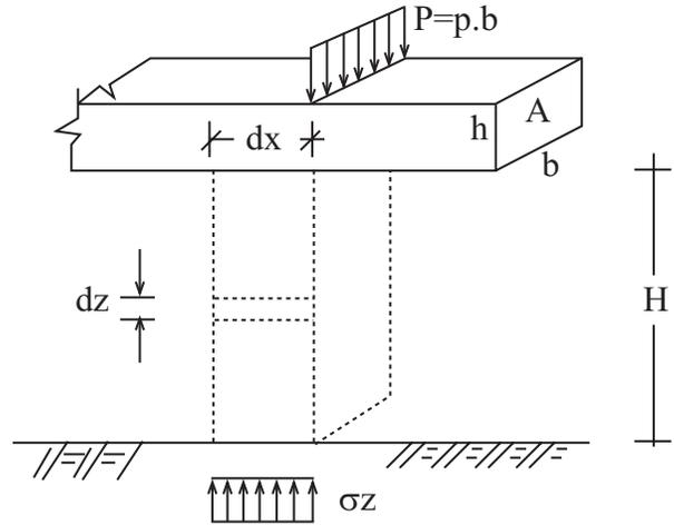
**Fig. (4).** Stress distribution under a beam of width  $b$ .
