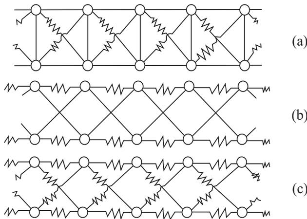
**Fig. (1).** Lumped mass and spring models with hinged joints for the wave travel properties: (a) Shear stiffness, and translation inertia only, (b) Flexural stiffness, and translation inertia only, and (c) Flexural and shear stiffness as well as translation and rotatory inertias.
