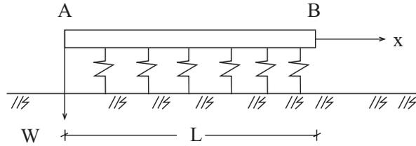
**Fig. (3).** Finite beam on elastic foundation.
