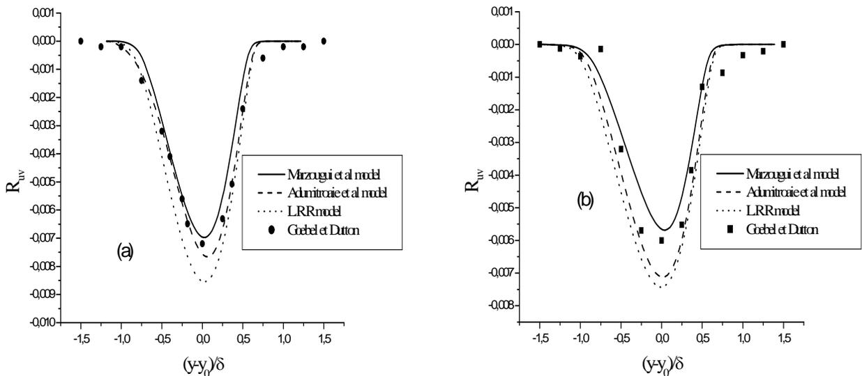
Fig. (4). Similarity profiles of Reynolds stress: (a)  $M_c = 0.69$ , (b)  $M_c = 0.86$ .
