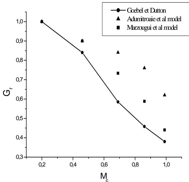
Fig. (6). Normalized growth rate  $G_r$  versus convective Mach number.
