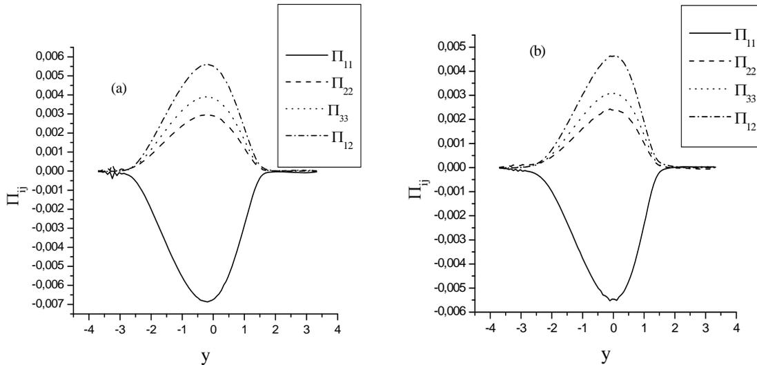
Fig. (5). Similarity profiles of pressure-strain correlation: (a)  $M_c = 0.69$ , (b)  $M_c = 0.86$ .
