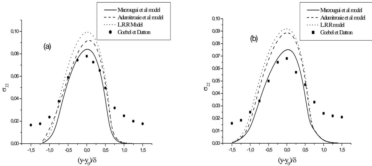
Fig. (3). Similarity profiles of transverse turbulence intensity: (a)  $M_c = 0.69$ , (b)  $M_c = 0.86$ .
