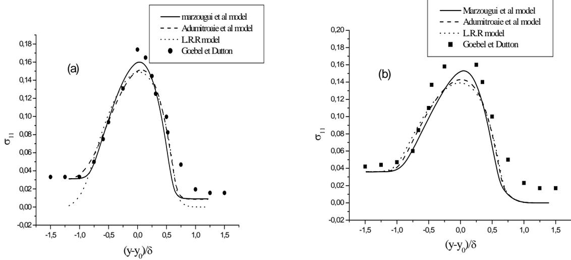
Fig. (2). Similarity profile of longitudinal turbulence intensity: (a)  $M_c = 0.69$ , (b)  $M_c = 0.86$ .
