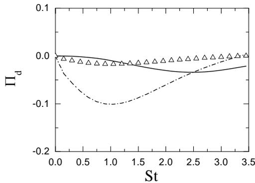
**Fig. (2).** Evolution of the pressure-dilatation correlation term  $\Pi_d$  for compressible homogeneous shear flow ( $M_{g0} = 48$ ). — : RDT prediction; ---: Hamba model before calibration;  $\Delta \Delta$  : Hamba model after calibration.
