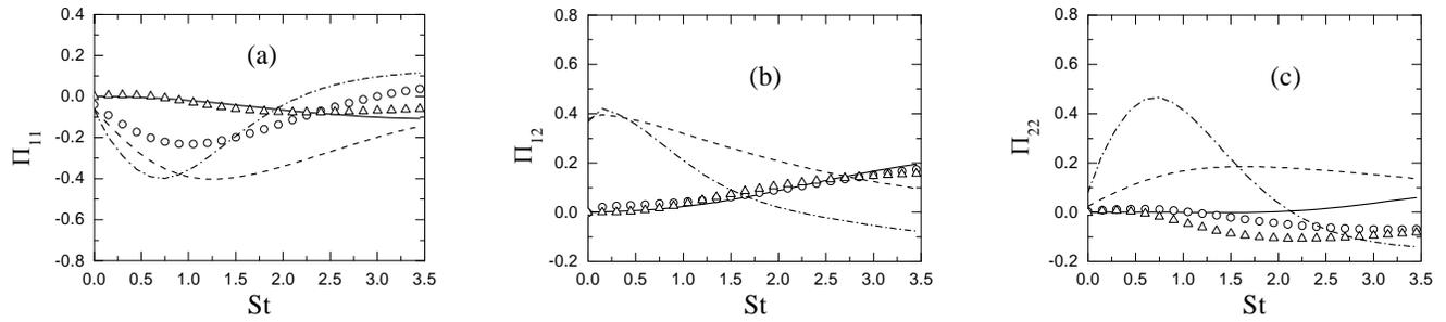
**Fig. (1).** Evolution of the pressure-strain correlations  $\Pi_{11}$  (a),  $\Pi_{12}$  (b) and  $\Pi_{22}$  (c) for compressible homogeneous shear flow ( $M_{g0} = 48$ ). — : RDT prediction; ---: Hamba model before calibration;  $\Delta \Delta$ : Hamba model after calibration; ---: Marzougui *et al.* model before calibration; o o: Marzougui *et al.* model after calibration.
