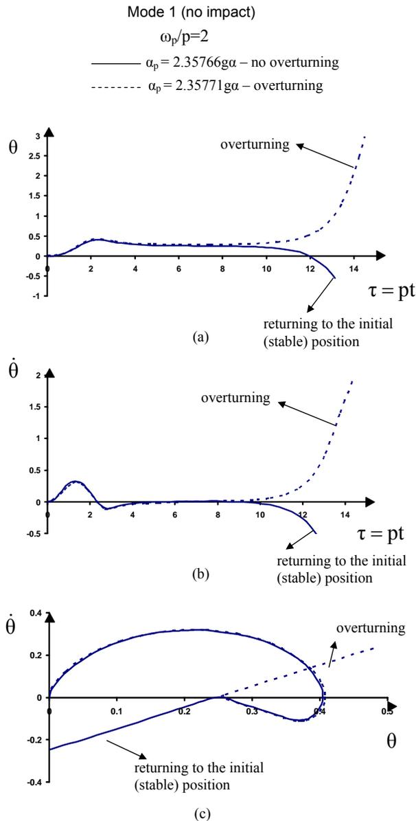
**Fig. (8).** Linearized solutions predicting the response of a rigid block (with  $p=2.14$ ,  $\alpha=0.25$  and  $\omega_p/p=2$ ) under one-sine pulse ground excitation presented as: (a)  $\theta$  versus  $\tau=pt$ , (b)  $\dot{\theta}$  versus  $\tau=pt$  (where  $\tau$  is dimensionless time) and (c) phase-plane portrait  $\dot{\theta}$  versus  $\theta$ .
