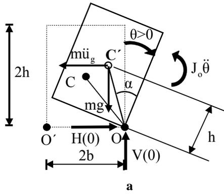
Fig. (4). a. Free body diagram of the block.
