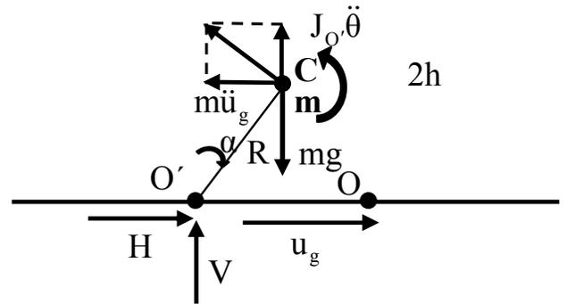
Fig. (5). Dynamic reactions acting on the point  $O'$  at the initiation of rocking motion ( $t=0$ ).
