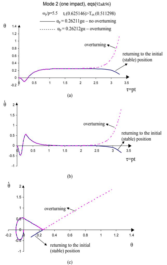
**Fig. (13).** Linearized solutions predicting the response of a rigid block with  $p=2.14$ ,  $\alpha=0.25$  and  $\omega_p/p=5.5$  ) under one-sine pulse ground excitation presented as: (a)  $\theta$  versus  $\tau=pt$ , (b)  $\dot{\theta}$  versus  $\tau=pt$  (where  $\tau$  is dimensionless time) and (c) phase-plane portrait  $\dot{\theta}$  versus  $\theta$ .
