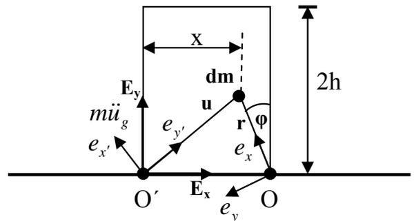
Fig. (7). Rectangular block under rocking motion just before it impacts on point O'.
