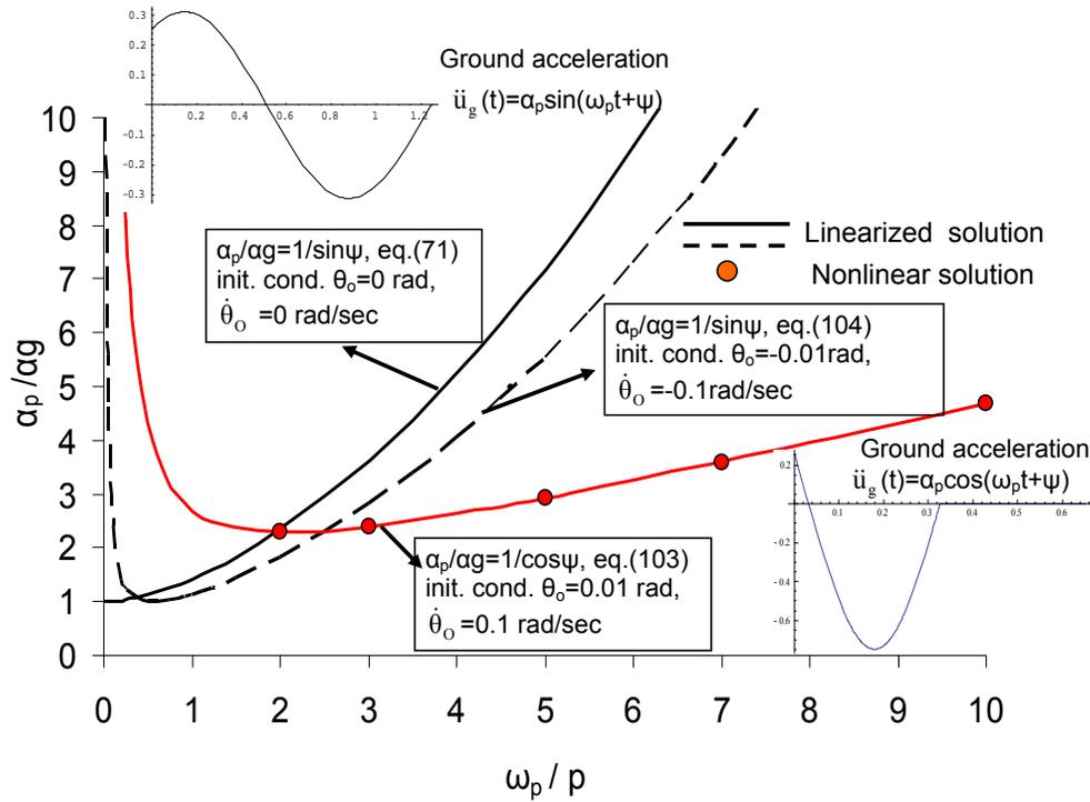
**Fig. (14).** The predicted values of minimum amplitude acceleration for overturning instability,  $\alpha_p/\alpha_g$  versus  $\omega_p/p$ , for the trivial initial conditions  $\theta_0 = \dot{\theta}_0 = 0$  and the nontrivial ones:  $\theta_0 = \pm 0.01$  rad,  $\pm \dot{\theta}_0 = 0.1$  rad/sec.
