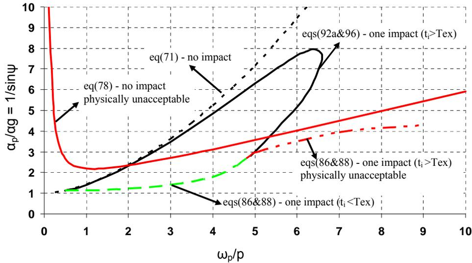
Fig. (10). The predicted values of minimum amplitude acceleration for overturning instability,  $\alpha_p/ag$  versus  $\omega_p/p$ .
