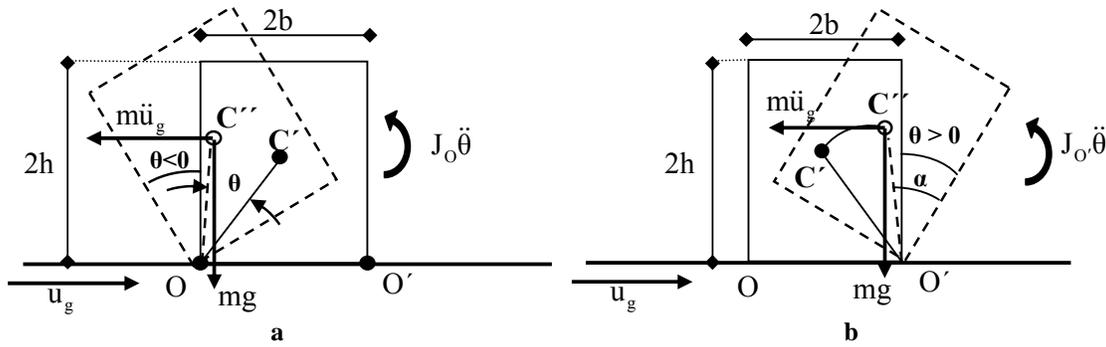
Fig. (3). a. Free body diagram of the block related to Fig. (2a), b. Free body diagram of the block related to Fig. (2b).
