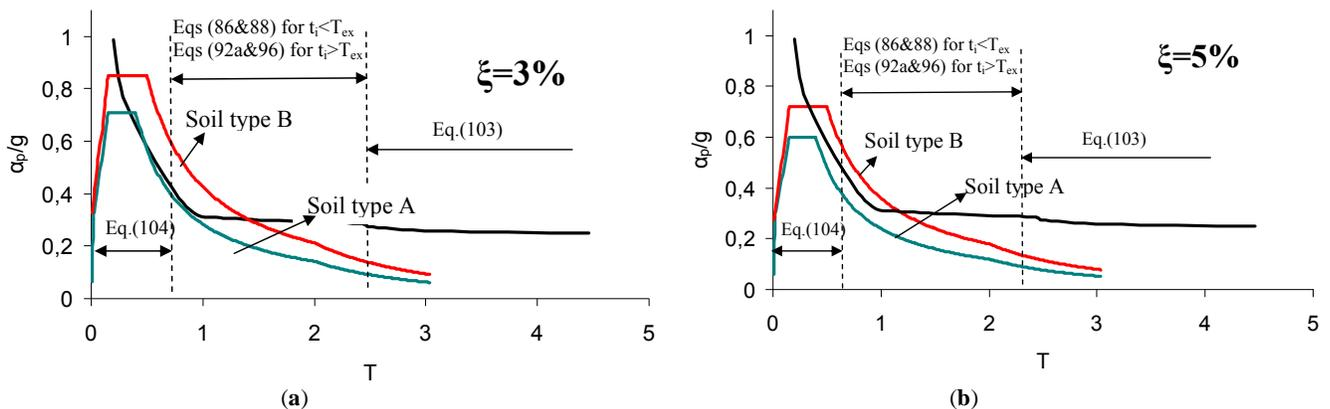
**Fig. (16).** Comparison of minimum amplitude acceleration  $\alpha_p/g$  versus  $T$  (period of forcing function) with the corresponding predictions of EC8 for two types of soil foundation (A and B) and damping: (a)  $\xi=3\%$  and (b)  $\xi=5\%$ .
