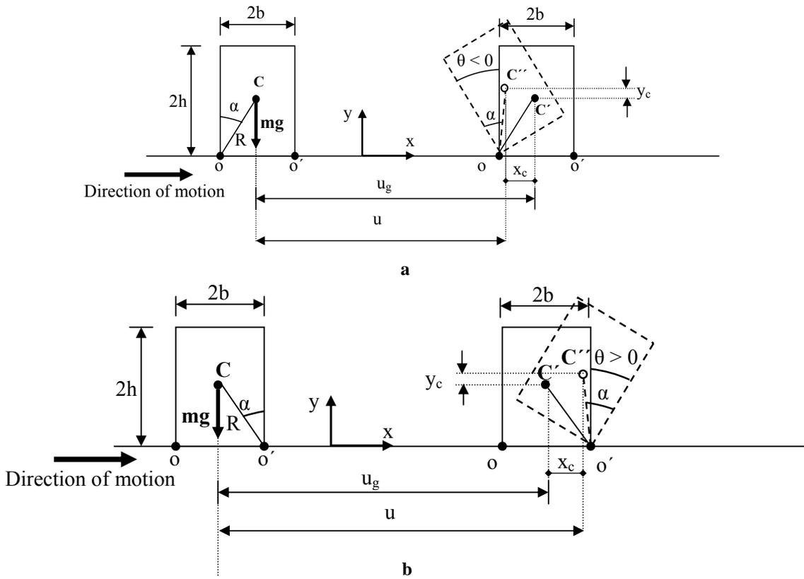
**Fig. (2).** **a.** Rigid body block displacement under ground excitation (rather suddenly applied), **b.** Rigid body block displacement under ground excitation (rather suddenly reduced).
