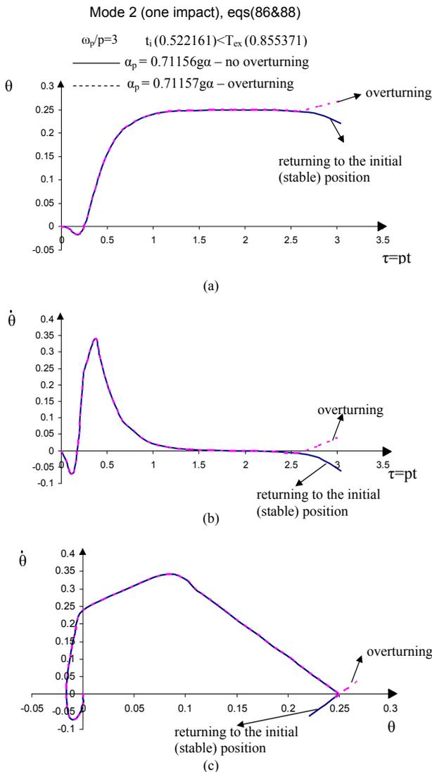
**Fig. (12).** Linearized solutions predicting the response of a rigid block (with  $p=2.14$ ,  $\alpha=0.25$  and  $\omega_p/p=3$ ) under one-sine pulse ground excitation presented as: (a)  $\theta$  versus  $\tau=pt$ , (b)  $\dot{\theta}$  versus  $\tau=pt$  (where  $\tau$  is dimensionless time) and (c) phase-plane portrait  $\dot{\theta}$  versus  $\theta$ .
