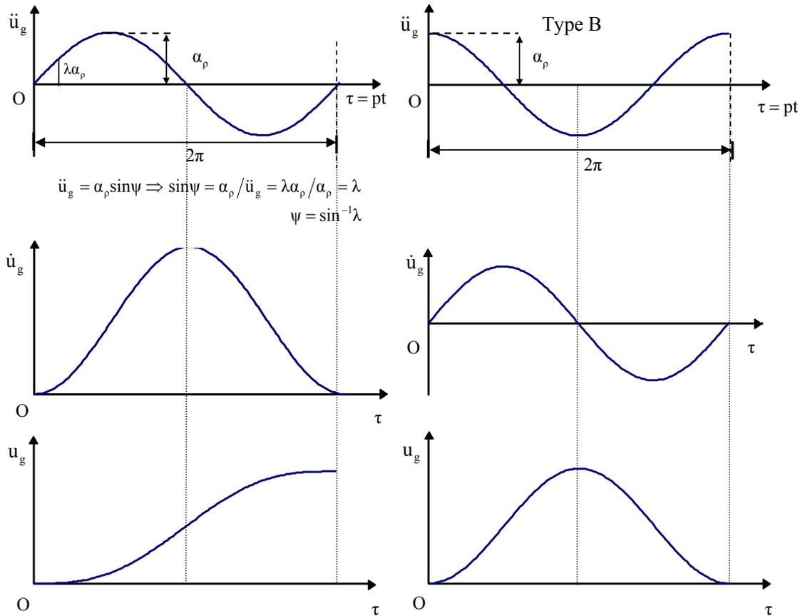
Fig. (6). Acceleration, velocity and displacement histories of one-sine (left) and one-cosine (right) pulse.
