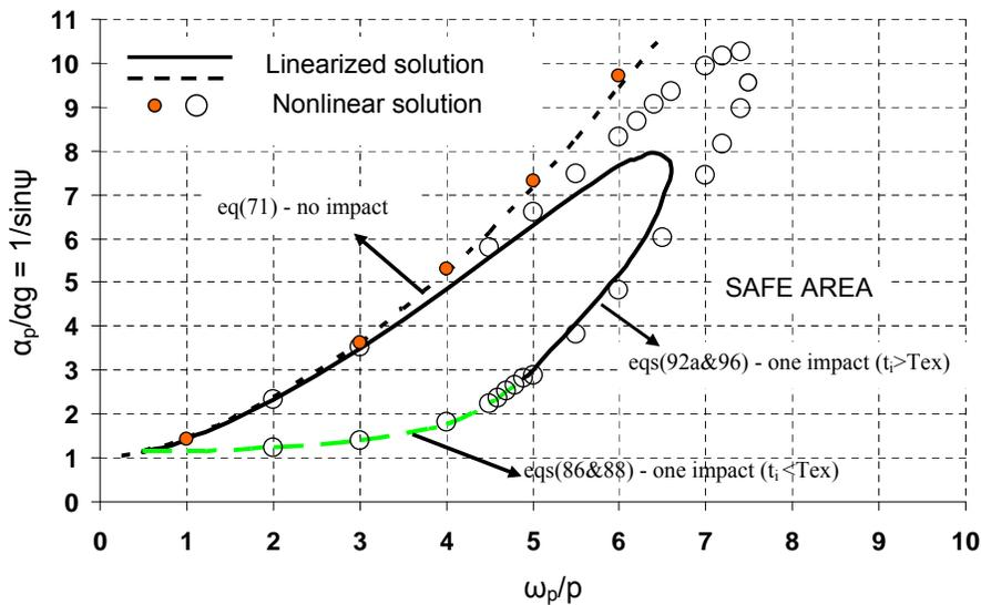
Fig. (11). Comparison of predicted values of minimum amplitude acceleration for overturning instability as obtained from the linearized solution and nonlinear analysis.
