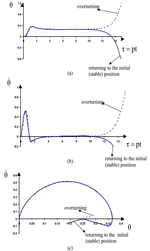
**Fig. (9).** Linearized solutions predicting the response of a rigid block (with  $p=2.14$ ,  $\alpha=0.25$  and  $\omega_p/p=4$ ) under one-sine pulse ground excitation presented as: (a)  $\theta$  versus  $\tau=pt$ , (b)  $\dot{\theta}$  versus  $\tau=pt$  (where  $\tau$  is dimensionless time) and (c) phase-plane portrait  $\dot{\theta}$  versus  $\theta$ .
