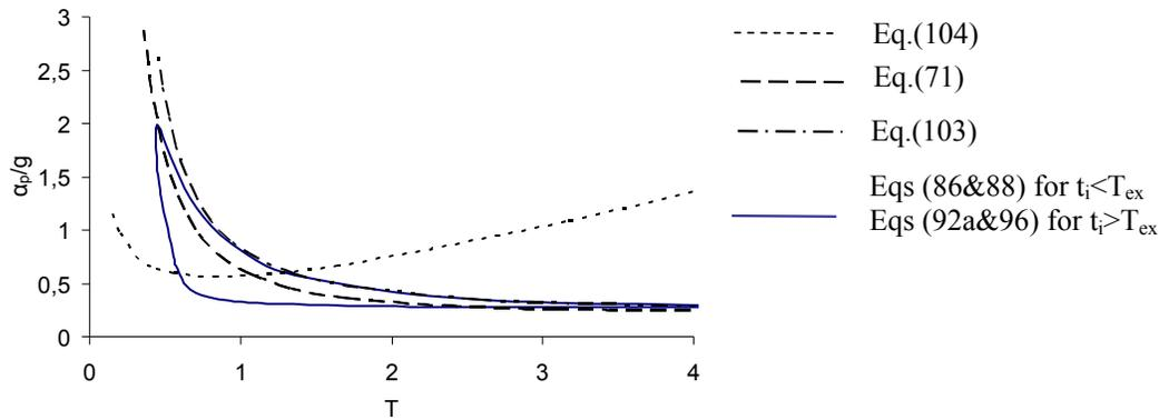
**Fig. (15).** Curves of minimum amplitude ground acceleration  $\alpha_p/g$  versus  $T$  (period of forcing function).
