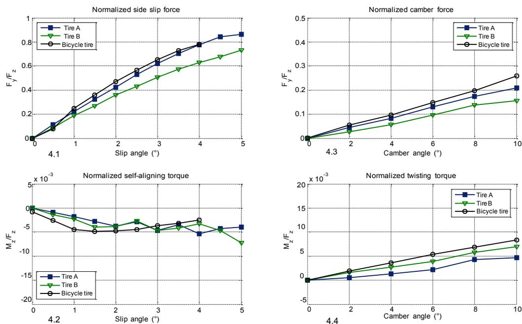
**Fig. (4).** Forces and torques of wheelchair and bicycle tires in reference conditions (vertical load 400 N, inflation pressure 4 bar and disc speed 4 km/h).
