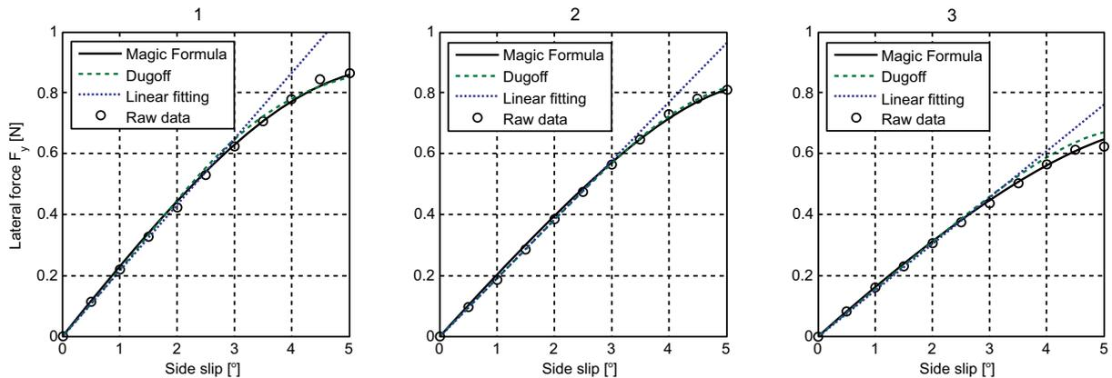
Fig. (8). Fittings of lateral force raw data by means of the Magic Formula and Dugoff models for tire A; (1) reference condition, (2) decreased inflation pressure, (3) increased load.
