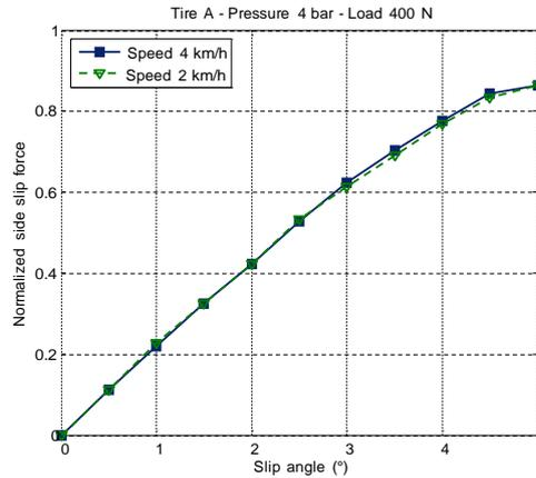
Fig. (5). Effect of forward speed on side slip force.
