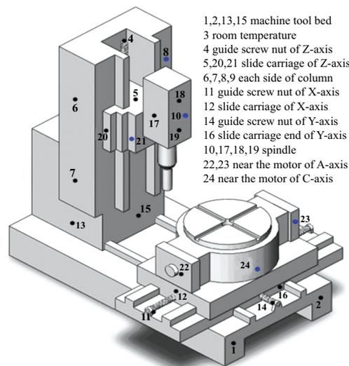
**Fig. (1).** Main thermal sources of a CNC machine tool.
