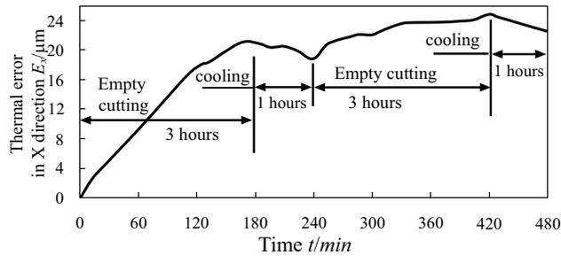
Fig. (4). Thermal errors in X-axis direction.
