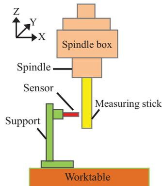
Fig. (3). Measurement of X-axis thermal errors.
