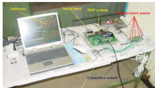
Fig. (5). Test system of thermal error model.
