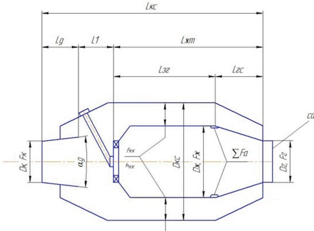
Fig. (1). Typical scheme and the main designations of external tubular CC.
