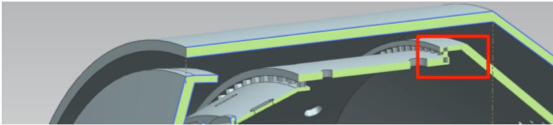
Fig. (12). FT case cracks.
