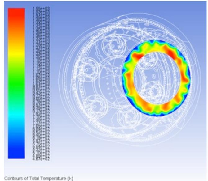
Fig. (15). Temperature field at CC outlet.
