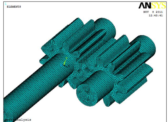
Fig. (3). FEA of gear mesh.
