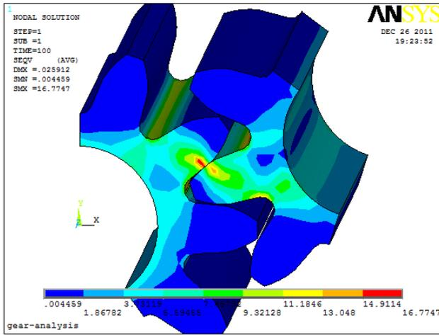
Fig. (4). Gear stress cloud chart.
