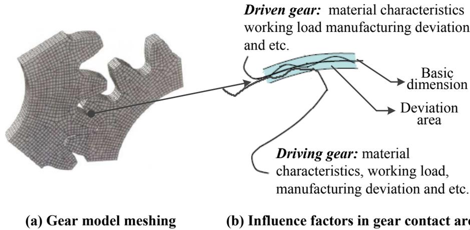
Fig. (1). Multi-factor influence on finite element analysis.
