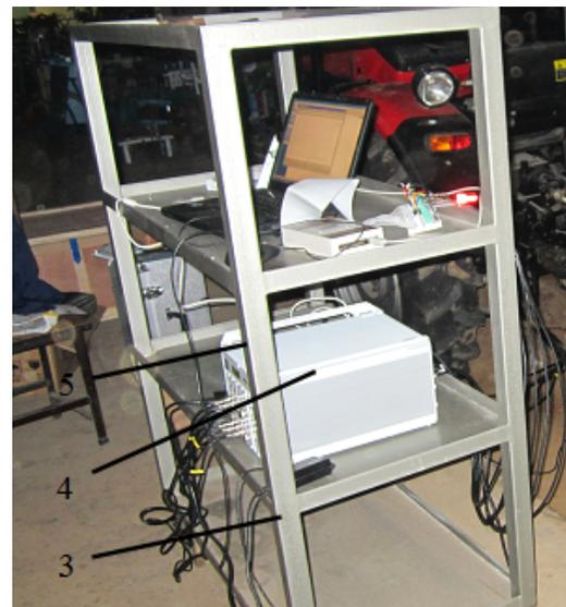
1-The force measuring device; 2-Vibratory subsoiler; 3-Dynamic strain gauge; 4-Data acquisition system; 5-Vibration test system
