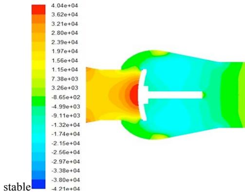
Fig.5 Pressure contour in shuttle check valve in the stable
