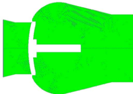
Fig.3 mesh map of shuttle valve model
