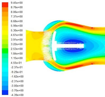
Fig.4 Velocity vector in shuttle valve in the
