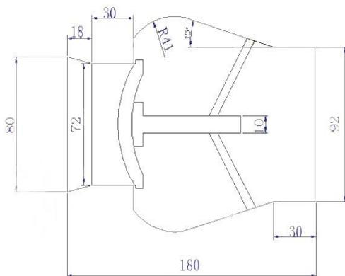
Fig.2 model diagram of shuttle valve
