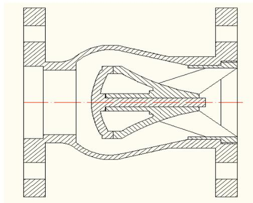
backpressure [10]. Functionally speaking, the shuttle check valve can function as opening and closing, throttling, damping, and amplify regulator and controller.
