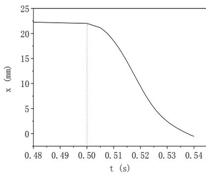
Fig. 9 The opening degree of valve spool in shuttle check valve during closing process
