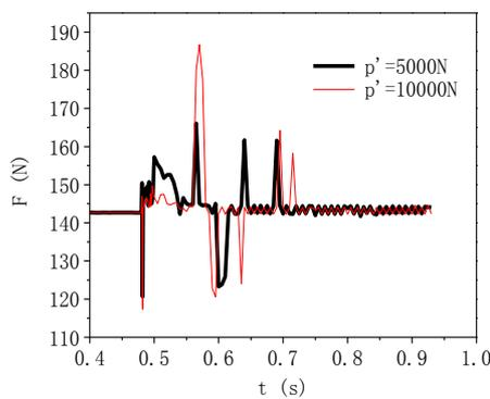
Fig.11 The curve of valve spool by fluid pressure in different pressure fluctuation
