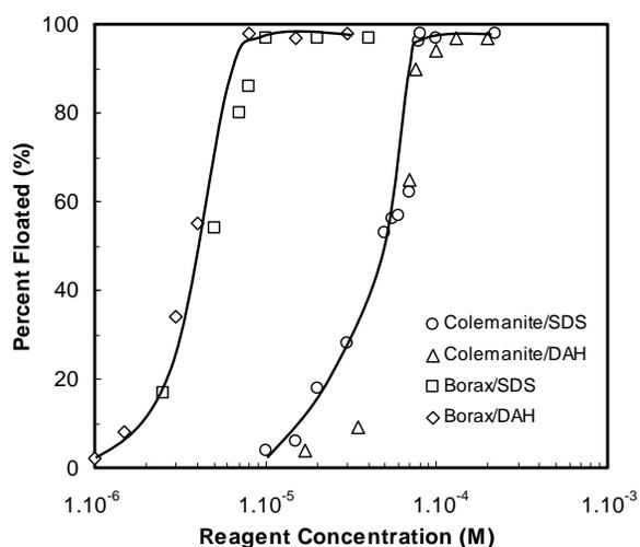
**Fig. (10).** Flotation recoveries of colemanite and borax vs. the concentration of anionic (SDS) and cationic (DAH) surfactants at pH 9.3 [18].
