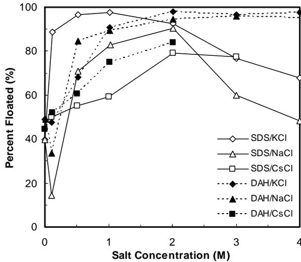
Fig. (12). Effect of monovalent salts on the flotation of colemanite with  $4.10^{-5}$  M of anionic (SDS) and cationic (DAH) collectors, pH  $9.3 \pm 0.1$  [16].
