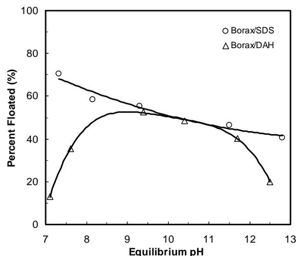
Fig. (9). Flotation of borax as a function of pH in the presence of anionic and cationic surfactants [18].
