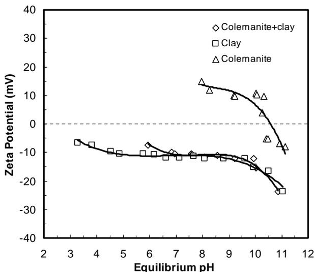
Fig. (7). Zeta potential of colemanite, clay and the mixture of colemanite and clay (1 g + 0.1 g) as a function of pH [16].
