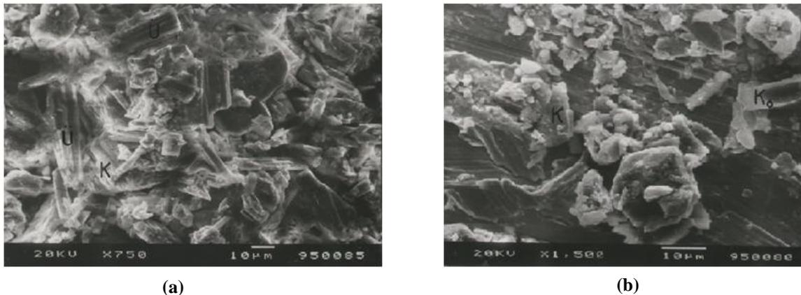
Fig. (19). SEM of (a) ulexite + clay mixture and (b) colemanite + clay mixture in the presence of SDS.
