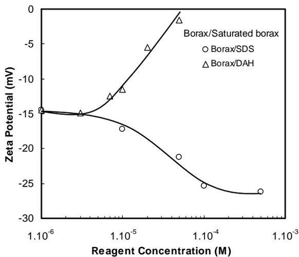
Fig. (5). Zeta potential of borax in the presence of anionic (SDS) and cationic (DAH) collectors at pH 9.3 [27].
