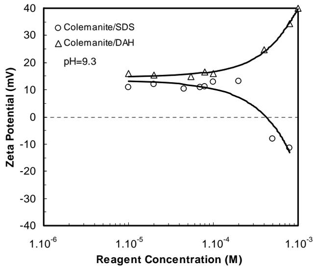
Fig. (4). Dependence of surfactant concentration on zeta potentials of colemanite at pH 9.3 [18].
