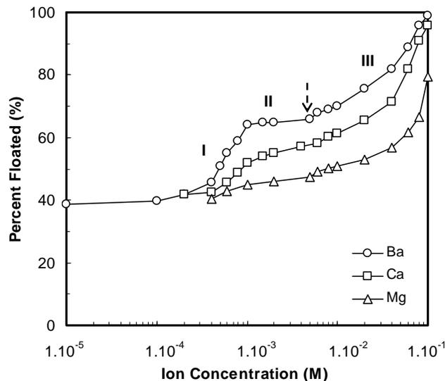
Fig. (13). Effect of multivalent ion concentration on the activation of colemanite at pH  $9.3 \pm 0.1$  [16].
