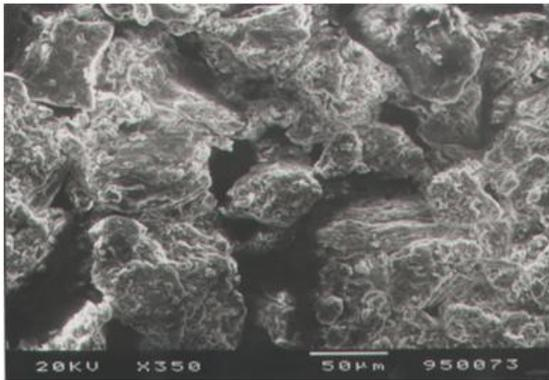
Fig. (18). SEM of clay in the presence of SDS.
