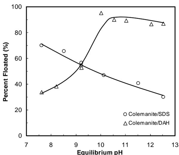
Fig. (8). Flotation of colemanite as a function of pH in the presence of SDS and DAH [18].
