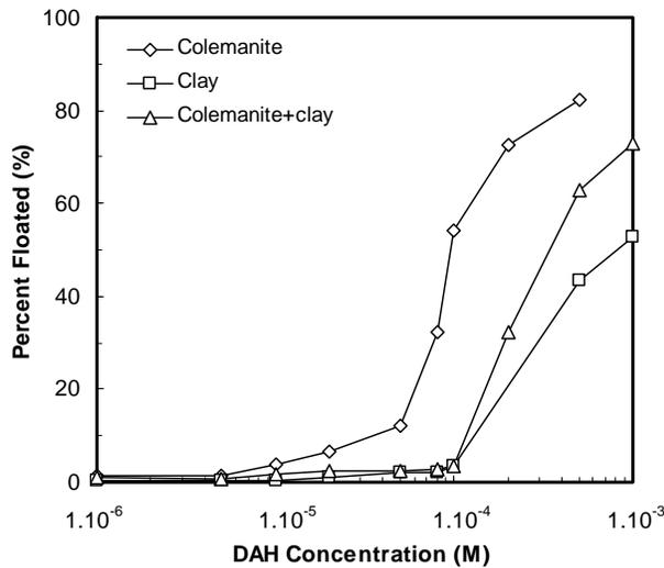
**Fig. (15).** Flotation of colemanite, clay, and colemanite+clay mixture as a function of DAH concentration at pH  $9.3 \pm 0.1$  (0.1% clay) [16].
