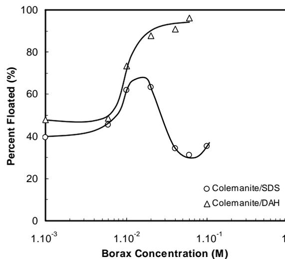
**Fig. (11).** Flotation of colemanite against borax with  $4.10^{-5}$  M concentration of SDS and DAH (pH 9.3) [27].
