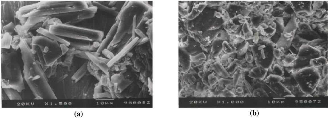
Fig. (17). SEM of (a) ulexite and (b) colemanite in the presence of SDS.
