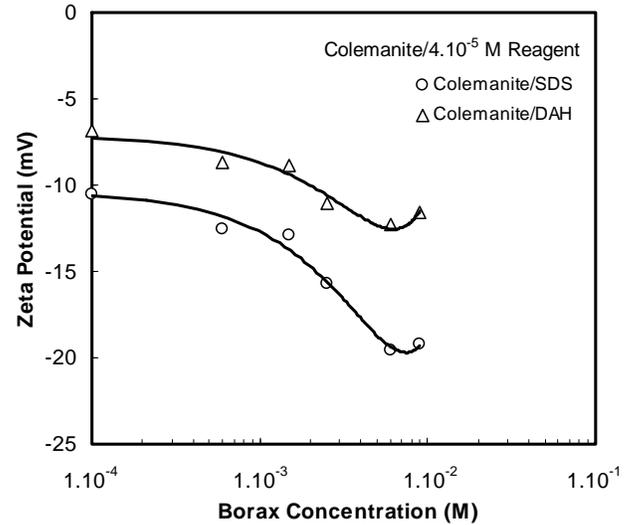
Fig. (6). Zeta potential of 1% by wt. colemanite against borax concentration in the presence of surfactants at pH 9.3 [27].
