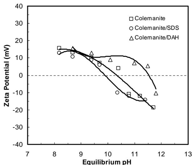
Fig. (3). Zeta potential of colemanite in the presence of surfactants [18].
