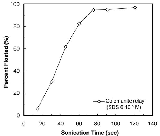
**Fig. (16).** In situ ultrasonic flotation for the colemanite/clay/SDS system as a function of sonication and flotation time at pH 9.3 [47].
