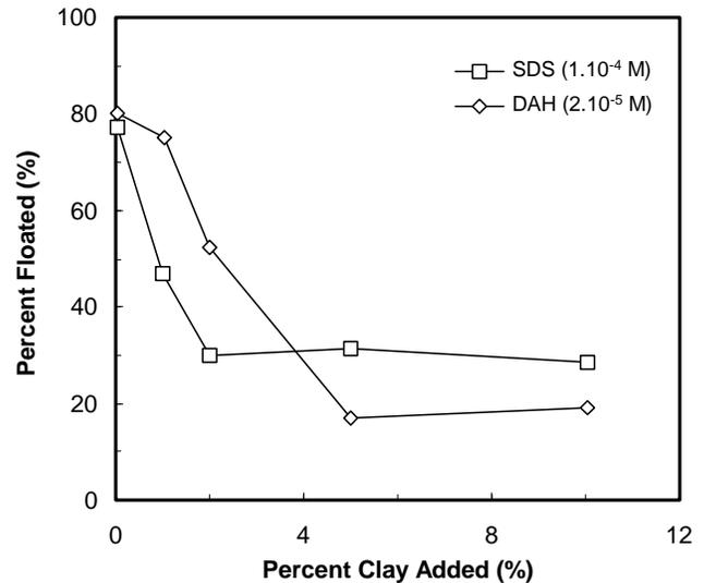
Fig. (14). Flotation of colemanite + clay mixture as a function of percent clay added in the presence of anionic (SDS) and cationic (DAH) collectors at the natural pH of 9.3 (The collectors were added into the mixture of colemanite and clay) [16].
