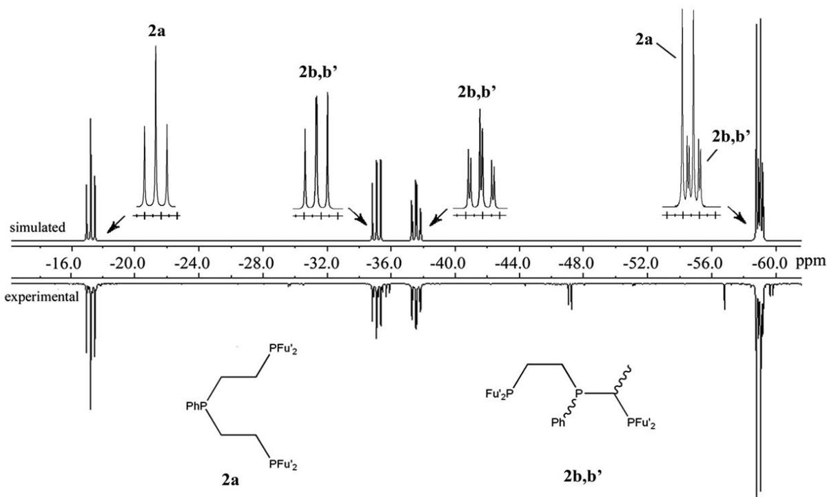
Fig. (1). Simulated and experimental <sup>31</sup>P{<sup>1</sup>H} NMR spectra of *Triphosfuranes 2*.
