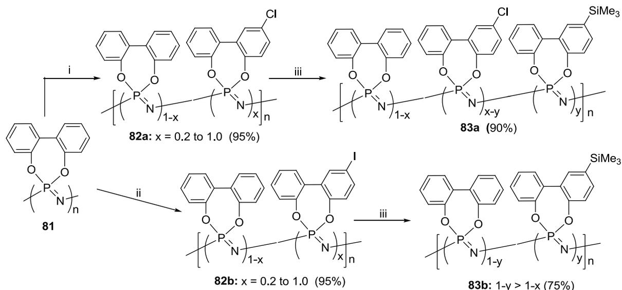
Reagents and conditions: (i)  $\text{Cl}_2/\text{H}_2\text{SO}_4$ ; (ii)  $[\text{Ipy}_2]\text{BF}_4/\text{HSO}_3\text{CF}_3$  in  $\text{Cl}_2\text{CH}_2$ ; (iii) 1,  $\text{LiBu}^t$  THF,  $-78^\circ\text{C}$ ; 2,  $\text{ClSiMe}_3$ .
