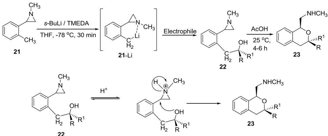
Scheme (6). Preparation of isochromans **23** *via* lithiation and acid-catalyzed cyclization.
