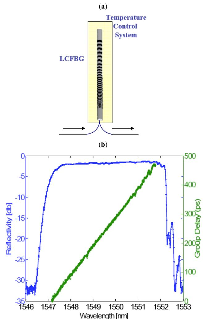
**Fig. (1).** Schematic view of the PTTD unit (a). LCFBG reflectivity and group delay of the LCFBG at  $30^\circ\text{C}$  (b).
