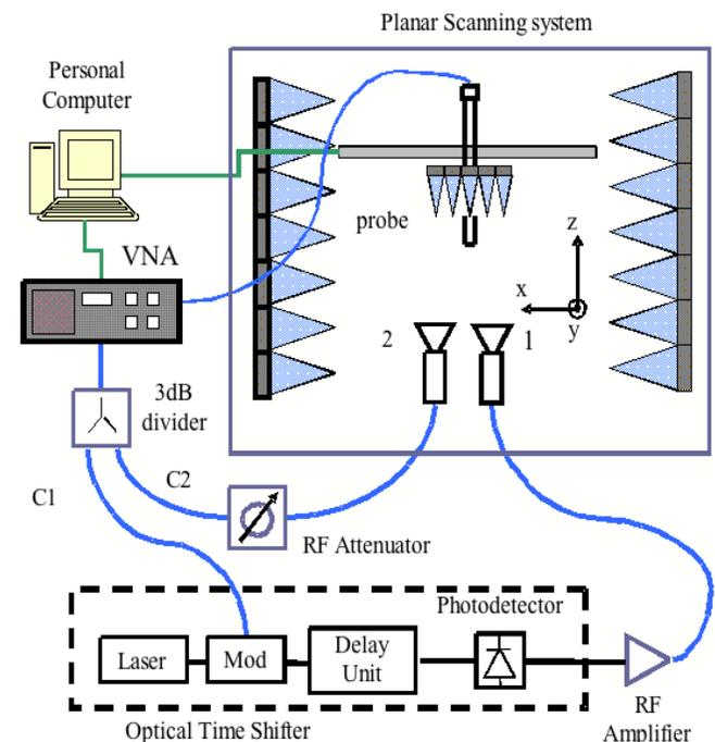
Fig. (4). Experimental setup for the beamsteering proof.
