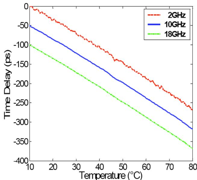
Fig. (2). Time Delay-Temperature characteristics of the TTD line retrieved at 2, 10 and 18GHz.
