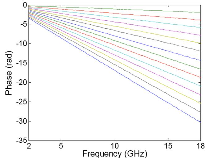
Fig. (3). Phase versus RF frequency for different set temperatures. Different lines correspond to different temperatures starting from  $T=10^\circ\text{C}$  and increasing up to  $T=80^\circ\text{C}$  in constant intervals of  $5^\circ\text{C}$ .
