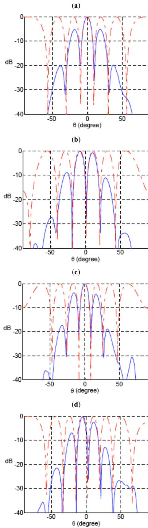
**Fig. (5).** Theoretical amplitude of the array factor (dashed line) and measured field pattern (solid line) at 15GHz for  $\theta_0=0^\circ$  (a) and  $\theta_0=10^\circ$  (b) and at 17GHz for  $\theta_0=0^\circ$  (c) and  $\theta_0=10^\circ$  (d).
