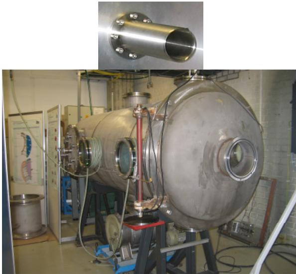
Fig. (13). Plasma accelerator and vacuum system.
