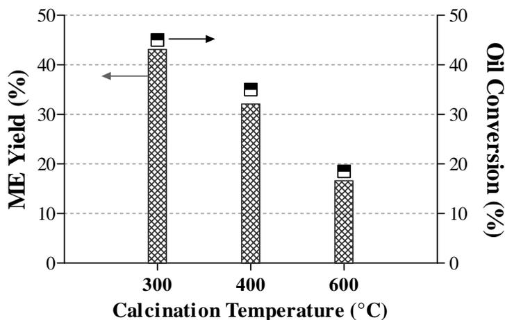
**Fig. (6).** Influence of the calcination temperature on ME yield (%) and oil conversion: sunflower oil weight, 80 g;  $R_{\text{met/oil}}$ , 12 mol/mol;  $R_{\text{cat/oil}}$ , 1 wt.%;  $T_R$ , 140°C; reaction time, 1 h.
