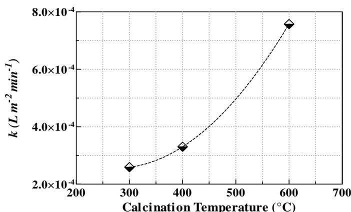
**Fig. (7).** Effect of the calcination temperature on reaction kinetics evaluated per unit of surface area: sunflower oil weight, 80 g;  $R_{\text{met/oil}}$ , 12 mol/mol;  $T_R$ , 140°C; reaction time, 1 h.
