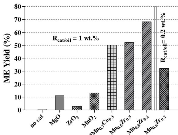
**Fig. (4).** ME yield (%) on Mn-based systems: sunflower oil weight, 80 g;  $R_{\text{met/oil}}$ , 12 mol/mol;  $R_{\text{cat/oil}}$ , 1 wt.%;  $T_R$ , 140°C; reaction time, 1 h (\*Ref. [21]).
