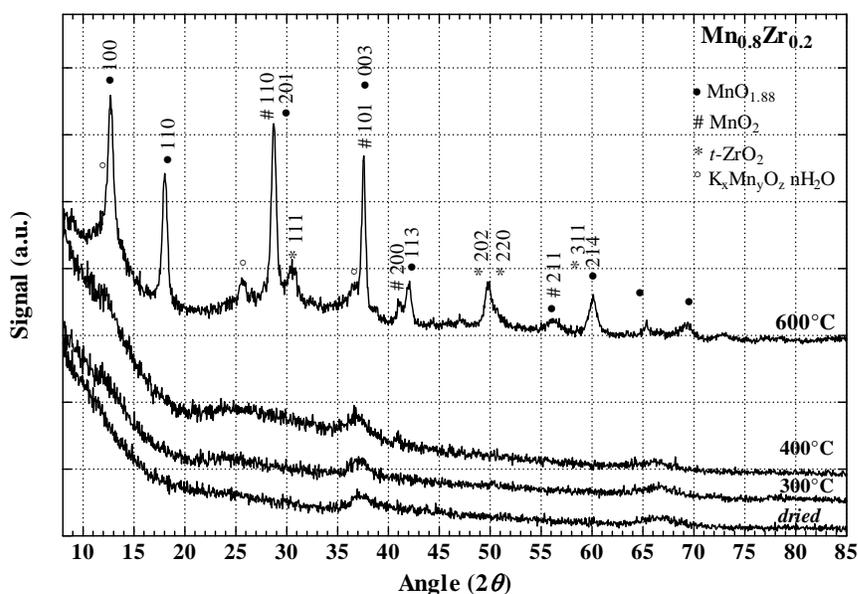
Fig. (2). Effect of the calcination temperature on the XRD pattern of Mn<sub>0.8</sub>Zr<sub>0.2</sub> sample.
