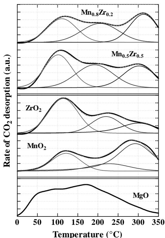
**Fig. (3).** CO<sub>2</sub> desorption profiles and deconvolution analysis in the range 0-350°C of the “bulk” oxides and MnZrO<sub>x</sub> samples.
