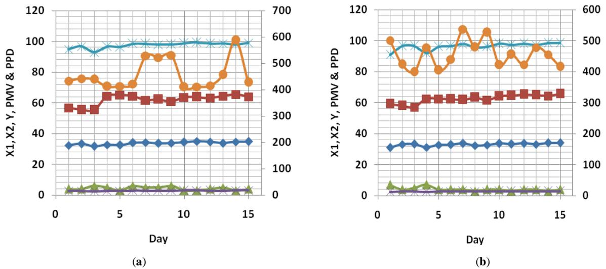
Fig. (11). Indoor RH, temperature, occupancy and CO<sub>2</sub> concentration for PMG Supermarket in the (a) morning; and (b) afternoon. Other details are as in Fig. (4).
