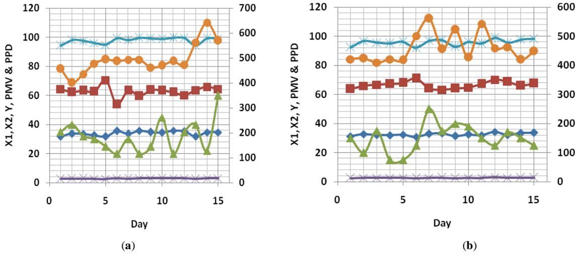
**Fig. (7).** Indoor RH, temperature, occupancy and CO<sub>2</sub> concentration for Eatery Hall in the (a) morning; and (b) afternoon. Other details are as in Fig. (4).
