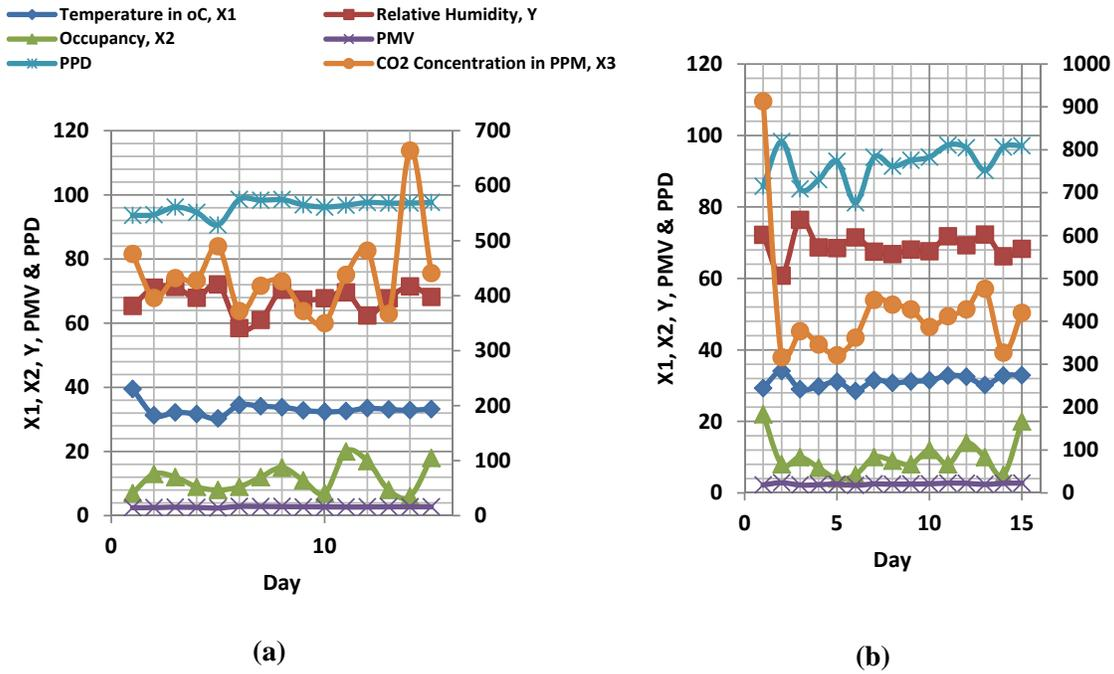
**Fig. (4).** Indoor RH, temperature, occupancy and CO<sub>2</sub> concentration for Husky Foods in the (a) morning; and (b) afternoon (The horizontal axis depicts the days, while the primary vertical axis depicts the temperature in degrees Celsius, relative humidity in %, occupancy, PMV and PPD; while the secondary vertical axis shows the CO<sub>2</sub> concentration in PPM).
