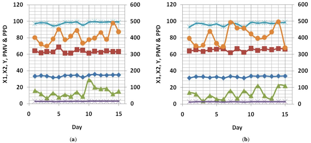
**Fig. (8).** Indoor RH, temperature, occupancy and CO<sub>2</sub> concentration for Wisdom Cafe in the (a) morning; and (b) afternoon. Other details are as in Fig. (4).
