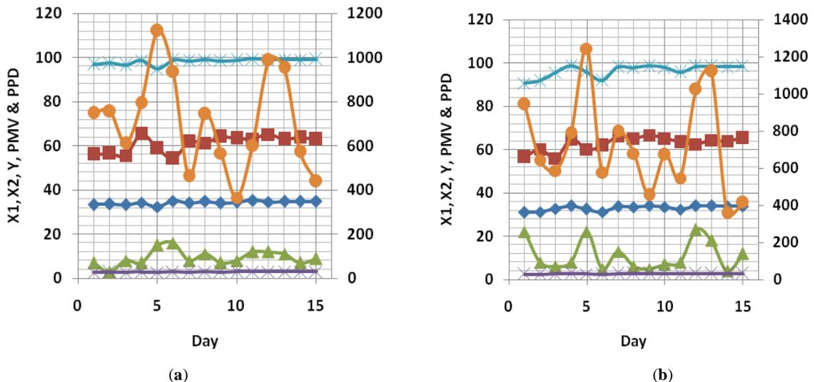
**Fig. (9).** Indoor RH, temperature, occupancy and CO<sub>2</sub> concentration for Pinto Lounge in the (a) morning; and (b) afternoon. Other details are as in Fig. (4).
