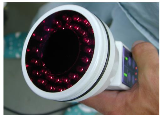
Fig. (3). External View of ICG fluorescence Imaging System (PDE).
