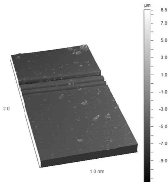
**Fig. (9).** Talystep 3D thin film thickness profile evaluation, 1x2 mm, corresponding to a representative sample, Co<sub>3</sub>O<sub>4</sub>/SS.
