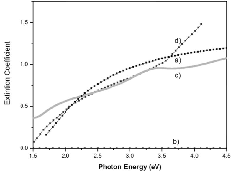
Fig. (4). Extinction coefficient of native oxides of the metal substrates: a) SS, b) Al, c) Fe and d) Cu.
