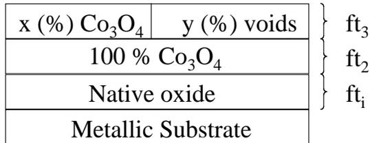
Fig. (5). Film layer structure that was employed to model the ellipsometric data. The  $ft_1$ ,  $ft_2$  and  $ft_3$ , stand for the thickness of the native oxide, the  $\text{Co}_3\text{O}_4$  solid film, and the mixed void–solid  $\text{Co}_3\text{O}_4$  film, respectively.
