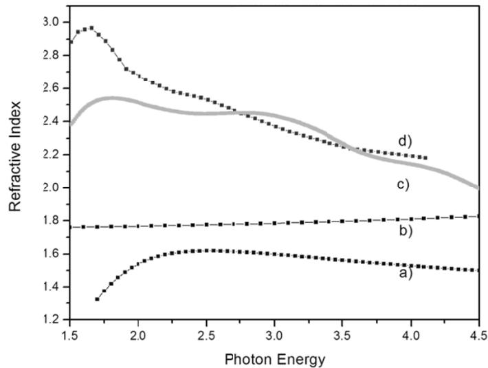
**Fig. (3).** Refractive index of native oxides of the metal substrates: a) SS, b) Al, c) Fe and d) Cu.
