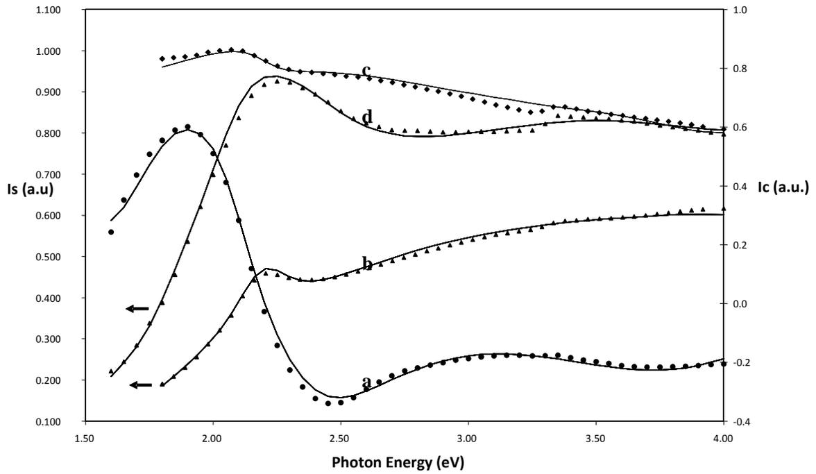
**Fig. (2).** Experimental (dotted line) and fitted (continuous line) ellipsometric parameters  $I_s$  and  $I_c$  vs photon energy plots of the uncoated copper substrate (a and b), and  $\text{Co}_3\text{O}_4$  – coated copper substrate (c and d).
