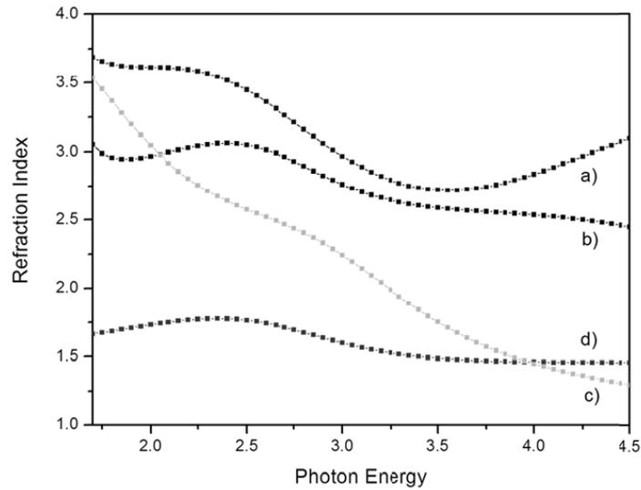
Fig. (6). Refraction index as a function of the photon energy (1.75–4.5 eV) of sol-gel deposited film on a) SS, b) Al, c) Fe and d) Cu. As indicated in the text, the film deposited on Fe is  $\text{CoFe}_2\text{O}_4$ , better than  $\text{Co}_3\text{O}_4$ .
