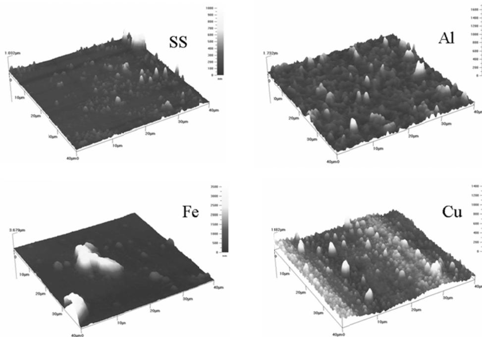
**Fig. (1).** AFM images of **a)** uncoated metal substrates (Fe = iron, SS = stainless steel, Al =aluminum, Cu = copper) and **b)**  $\text{Co}_3\text{O}_4$ - coated substrates.
