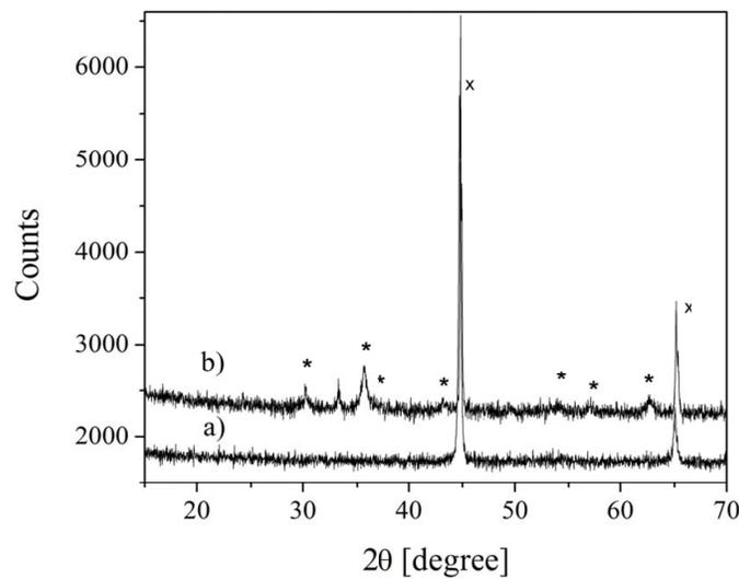
**Fig. (8).** X-ray diffractograms of the Iron substrate a) and the Iron substrate coated with Co<sub>3</sub>O<sub>4</sub> after heat treatment b). The peaks marked with an (x) correspond to iron (PDF 04-007-9753), and those identified with a (\*) correspond to CoFe<sub>2</sub>O<sub>4</sub> phase (PDF 04-016-3954).
