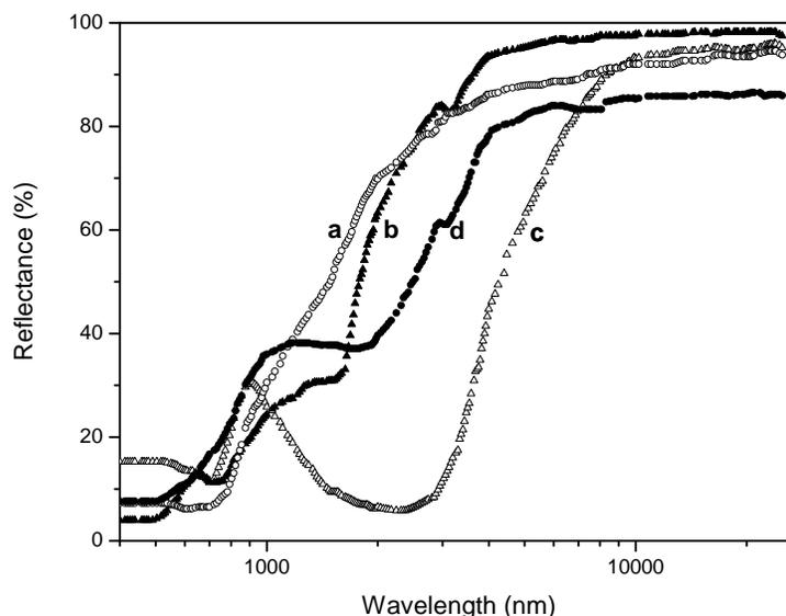
**Fig. (10).** UV – Vis IR reflectance spectra of the  $\text{Co}_3\text{O}_4$ /metal structures: a) SS, b) Al, c) Fe and d) Cu. The measurements were carried out in the 200 – 25000 nm wavelength range.
