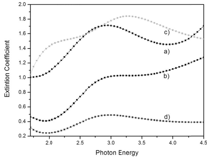
**Fig. (7).** Extinction coefficient as a function of the photon energy (1.75 – 4.5 eV) of sol-gel deposited film on a) SS, b) Al, c) Fe and d) Cu.
