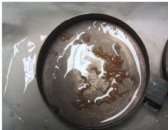
**Fig. (3).** CHI in 1.5% acetic acid dissolution loaded with PEG (1g) and submitted to 120°C for 45 min sterilization process.
