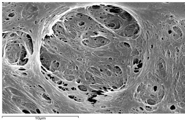
**Fig. (6).** SEM micrograph of TPP/CHI nanoparticles loaded with PEG (CHI 0.3 g/100 ml, TPP 0.1 g/100 ml and PEG 0.5 g/100 ml). The line for the scale denotes 10  $\mu$ m.
