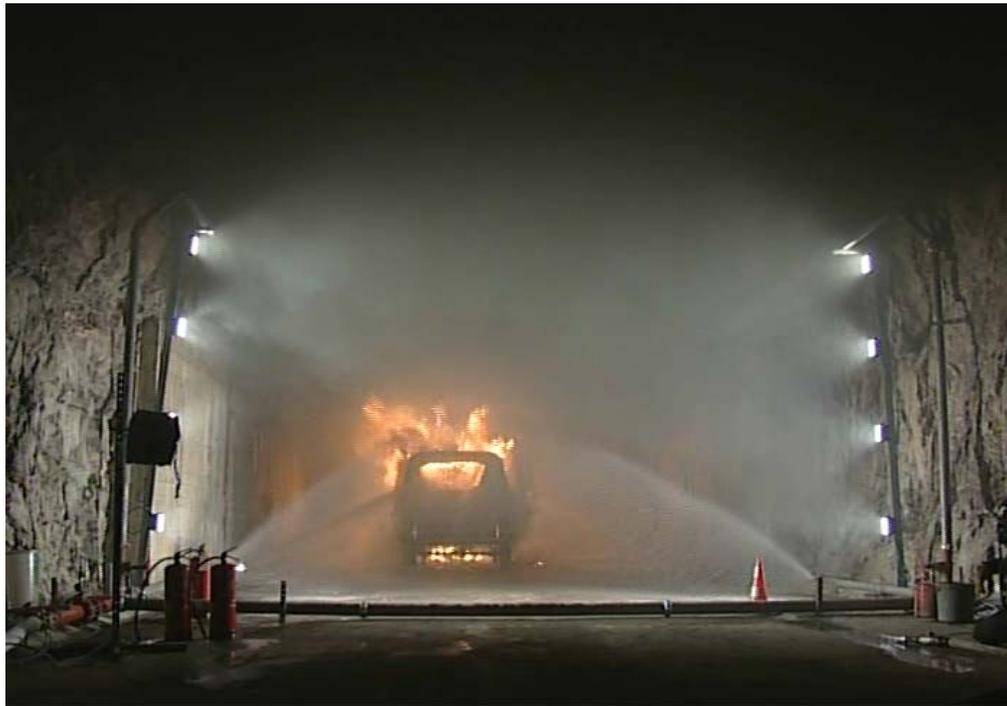
Fig. (7). Burning van and activation of the mitigation system in the Rosa tunnel.
