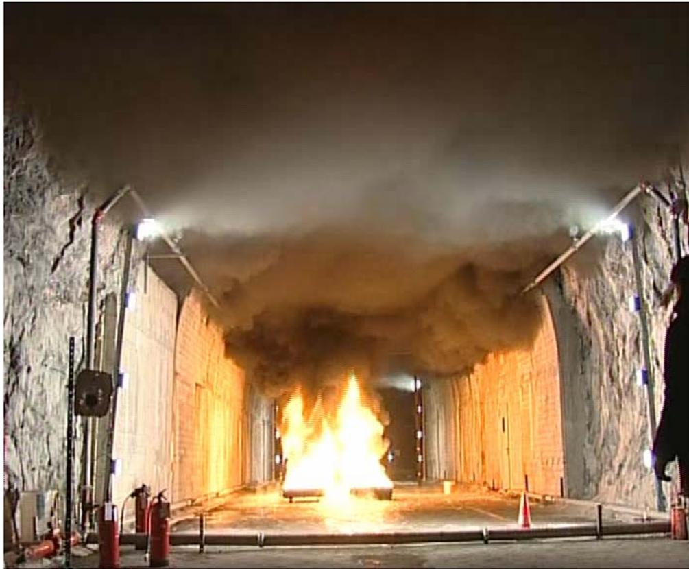
Fig. (5). Smoke stratification during a pool fire test in the Rosa tunnel.
