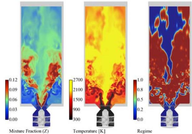
**Fig. (3).** LES of NASA's LDI spray combustor. Left: Filtered mixture fraction field. Middle: Filtered temperature field. Right: Filtered combustion regime indicator (see section 3.5) with red representing premixed and blue representing non-premixed combustion.
