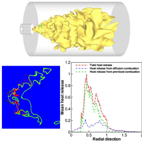
**Fig. (1).** DNS of a spray combustor from Ref. [12]. Top: Temperature isocontour in the combustor. Bottom Left: Flame index in combustor cut plane (see section 3.5), with red representing premixed and green representing non-premixed combustion. Bottom Right: Azimuthally integrated premixed, non-premixed, and total heat release in a cross section of the domain. Heat release is normalized by its maximum value, and the radial coordinate is normalized by the inlet pipe diameter.
