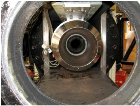
Fig. (1). Axisymmetric scramjet (upstream view).
