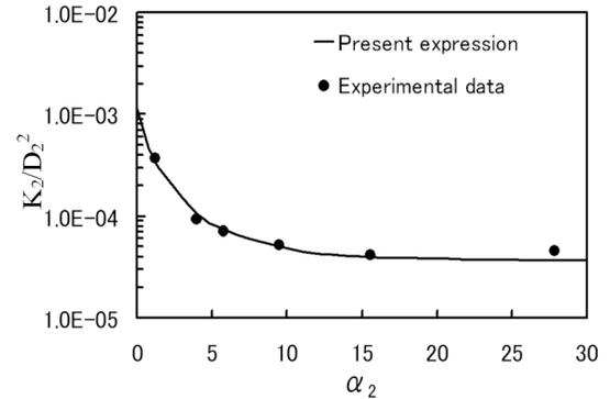
Fig. (4). Variation of effective permeability for the case of  $D_1 = 0.5$  mm and  $D_2 = 2.3$  mm.
