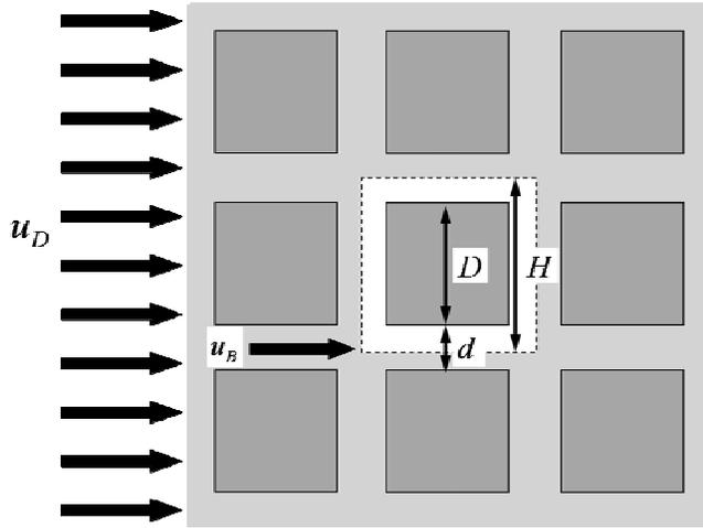
**Fig. (1).** Mathematical model having both vertical and horizontal fractures.
