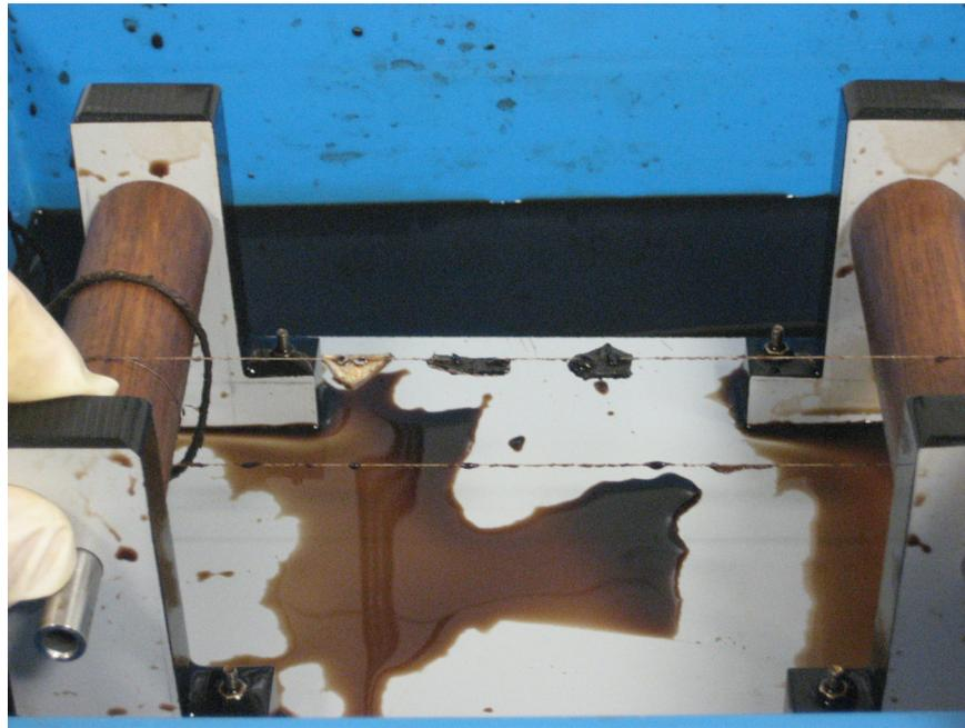
Fig. (1). Experimental set-up for simulation of moving particles in the black ferrofluid.
