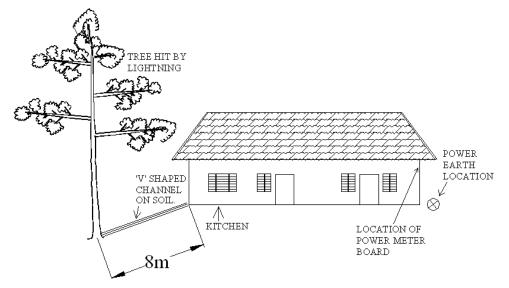
Fig. (3). Side view of the accident site of G3 indicating the tree hit by lightning and position of 'v' shaped channel on the soil. The tree was an isolated one.
