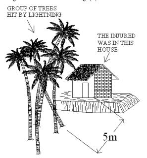
**Fig. (1).** Lightning accident through ground conduction from an isolated group of coconut trees to a house which had electric power wiring. Only these trees were present at the time of accident.
