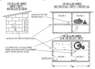
**Fig. (12).** Side view, vertical sectional view and plan view of the storage shed which was involved in lightning by ground conduction at site G19. The holes on the outside wall of Room 1 and the wall of the inside room namely Room 2 are shown.
