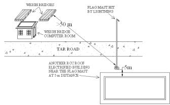
**Fig. (17).** Plan view of the accident site G24. The flag mast which was hit by lightning, the weigh bridges and the computer room can be seen.
