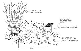
**Fig. (8).** The scene of the G13 accident. The position of the hole on the wall of the house is indicated. The fatally injured victim was on the other side of the wall. The bamboo bunch was not the only tree in the vicinity.
