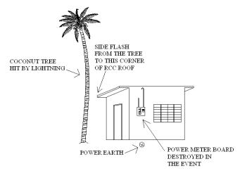
**Fig. (6).** Drawing of the site G11 showing the isolated coconut tree which was hit by lightning and the close by RCC building. The building and personnel inside were involved by side flash and ground conduction.
