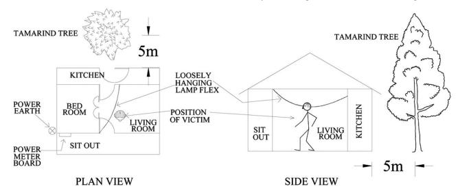
Fig. (2). Plan and side views of the G2 accident site showing the position of the victim at the time of lightning strike. Lightning hit the tamarind tree. Location of power earth is shown in plan view.
