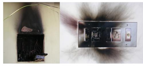
**Fig. (16).** The damaged Main Power Board (MB) of the house at location G23 is shown in photograph on the left and that of the Switch Board (SB) is shown on the right. It is clear that there was an explosion under SB panel.
