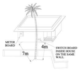
**Fig. (15).** The G23 location of accident. Power earth, power meter board and location of the switch board inside the house are shown.
