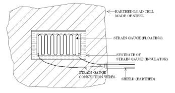
**Fig. (18).** Illustration of electrical nature of one load cell of a weigh bridge and strain gauge. Wires of the strain gauge going through a shielded cable is also shown.
