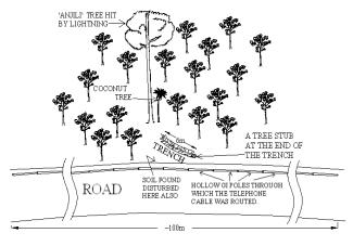
**Fig. (13).** Depiction of the lightning accident site G21. Heavy lightning current due to the presence of a chain of galvanised iron (GI) poles of about 100m length and telephone wires to several houses resulted in formation of a trench of 6 m length on soil.
