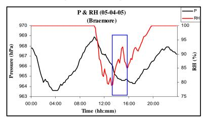
**Fig. (10).** P and RH variation at Braemore on 5<sup>th</sup> April 2005 which was a thunder storm day. A rectangular marker indicates the not so conspicuous depression and a corresponding significant change in RH.
