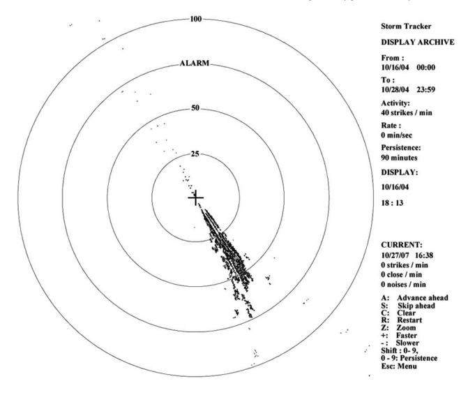
Fig. (5). Lightning detector display at 18:13 h on 16/10/04 showing thunderstorm activity for the past 90 minutes. Each dot indicates a lightning discharge event.
