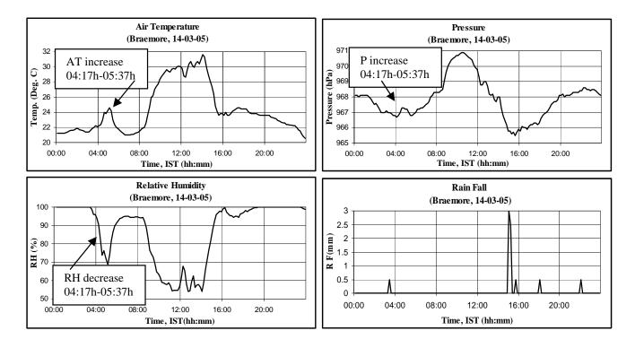
Fig. (2). Data on four weather elements from Braemore for 24 hours on 14/03/05 showing occurrence of atmosphere effect between 04:17 h and 05:37 h.
