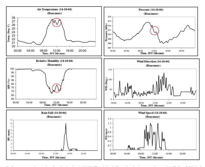
Fig. (6). Braemore weather station data for the day 14/10/04. The circles indicate the simultaneous changes in AT, P and RH during an updraft.
