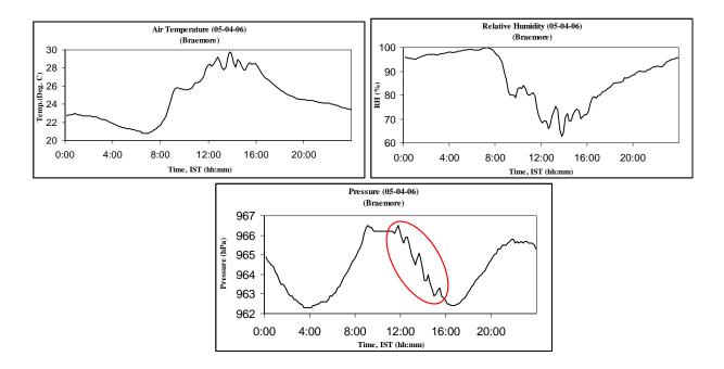
**Fig. (16).** Graphs of weather elements monitored at Braemore on 05/04/06 showing several updrafts between 1200h and 1600h. The elliptical marker is used to indicate several updraft events.
