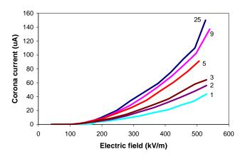
**Fig. (3).** The corona current as a function of the background electric field from clusters of needles. The number of needles in the cluster is shown in the diagram.
