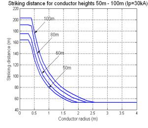
Fig. (6b). Striking distance for various conductor heights from 50m-100m with  $I_{peak}$ =30kA.
