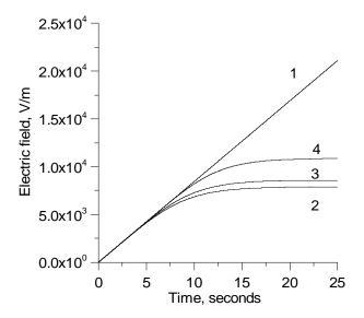
**Fig. (1).** The electric field at ground level produced by a thundercloud in the absence (curve 1) and in the presence (curves 2, 3 and 4) of ground corona. The threshold for corona inception is (2) 1kV/m, (3) 2 kV/m and (4) 5 kV/m.
