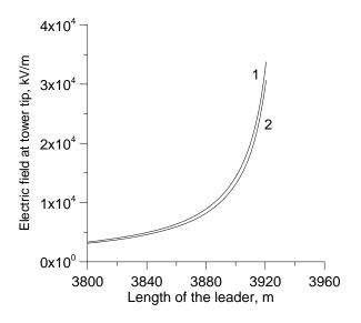
Fig. (7). The evolution of the electric field at the top of a 60 m tower located below the stepped leader trajectory as the stepped leader propagates towards the ground. Curve (1) shows the evolution of the electric field in the absence of space charge and the curve (2) depicts the electric field in the presence of space charge. The radius of the tower tip is 2 m.
