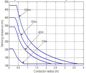
Fig. (6d). Striking distance for various conductor heights with  $I_{\text{peak}}$ =80kA.
