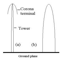
Fig. (5). (a) The tower and the corona terminal. (b) The semiellipsoid representing the complex body.
