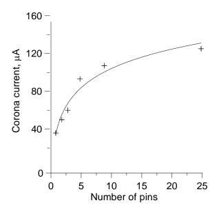
Fig. (4). The corona current at 500 kV/m as a function of the number of needles in the cluster.
