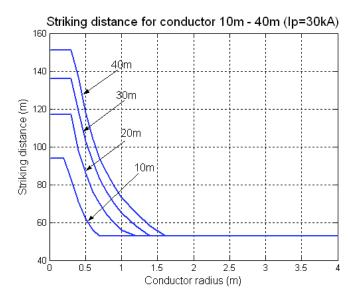
Fig. (6a). Striking distance for various conductor heights from 10m-40m with  $I_{peak}=30kA$ .
