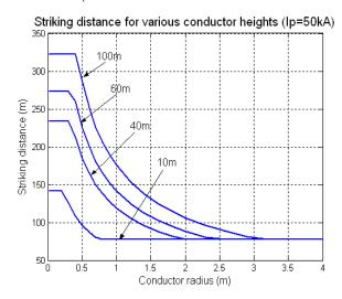
Fig. (6c). Striking distance for various conductor heights with  $I_{\text{peak}}$ =50kA.
