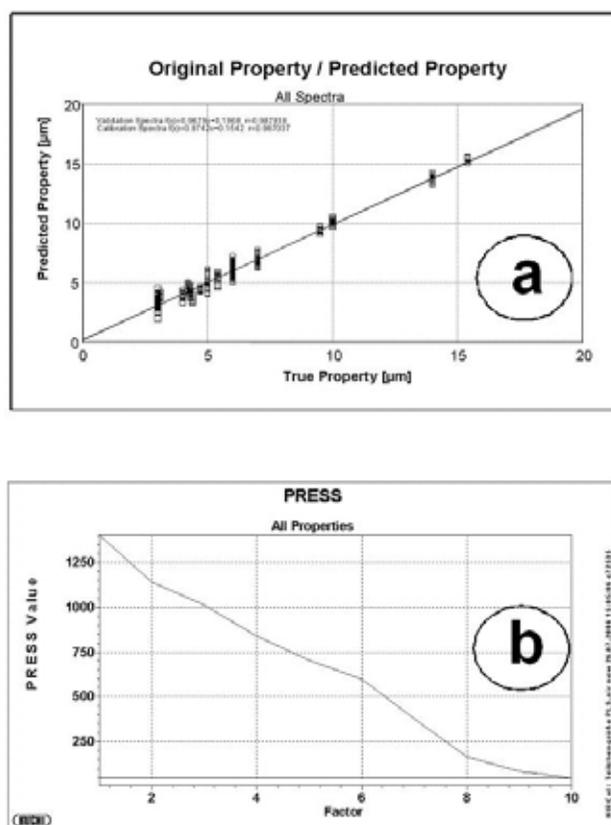
**Fig. (6).** (a) Predicted (NIRS) versus reference property for the determination of particle diameter; (b) PRESS (Predicted Residual Sum Square). Conditions: Data pre treatment, normalization by closure, first derivative BCAP (4440 - 9000  $\text{cm}^{-1}$ ); scans, 10; reflectance; temperature, 23 $^{\circ}\text{C}$ .
