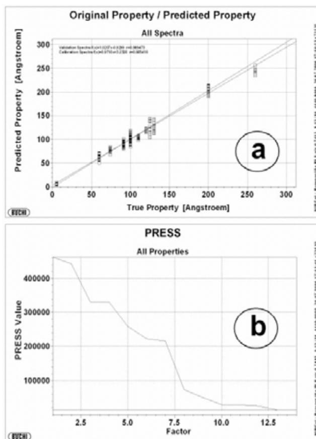
**Fig. (7).** (a) Predicted (NIRS) versus reference property for the determination of pore diameter; (b) PRESS (Predicted Residual Sum Square). Conditions: Data pre treatment, first derivative, normalisation by closure ( $4440\text{-}9000\text{ cm}^{-1}$ ); scans, 10; reflectance; temperature,  $23^\circ\text{C}$ .
