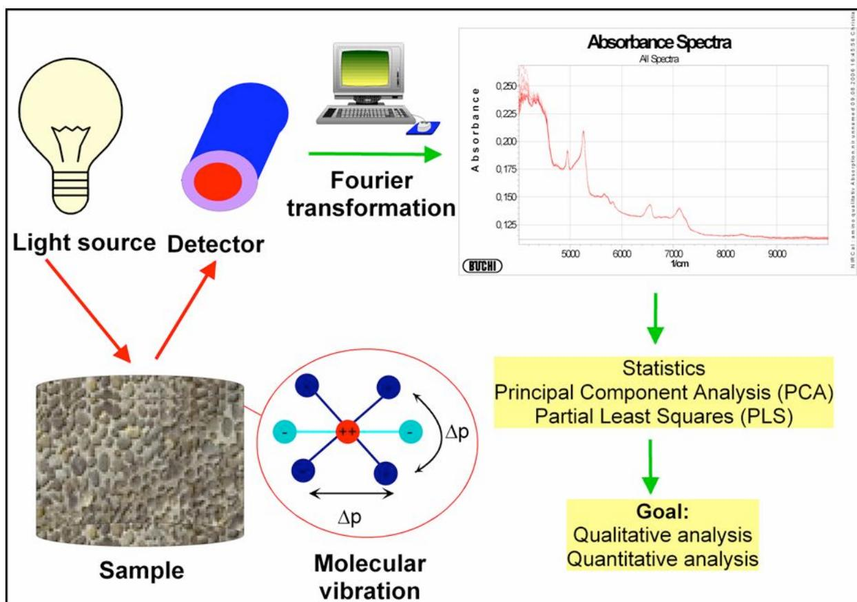
Fig. (3). Analytical workflow in near infrared reflection spectroscopy (NIRS).
