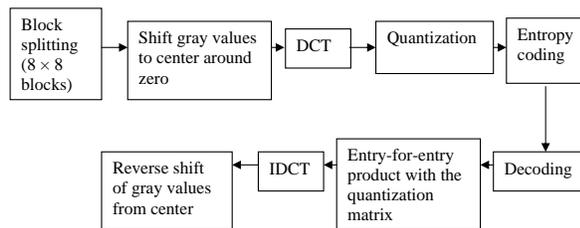
Fig. (1). The JPEG procedure.
