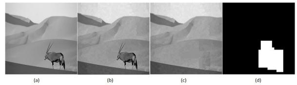
**Fig. (9).** (a) The original donkey image, (b) the watermarked image using variable-length chromosome algorithm with  $PSNR=41.14$ , (c) the CP-attacked image, and (d) the authentication image.
