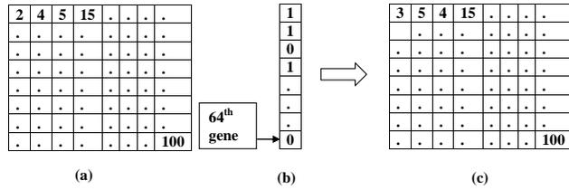
Fig. (5). (a) original 8x8 block, (b) 64-bit chromosome, and (c) adjusted block after substituting (b) in (a).
