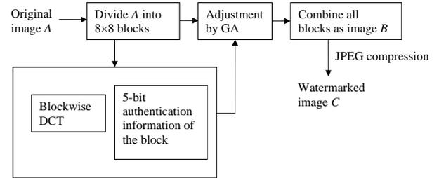
Fig. (2). The overall watermark embedding procedure.
