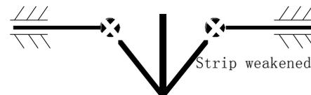
**Fig. (1).** the localize deformation under point load for partially cut-out blank.
